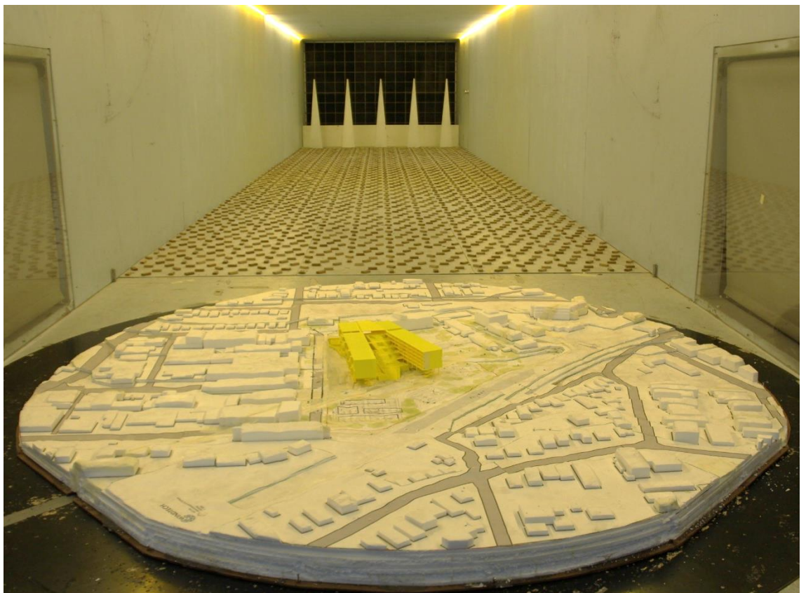
Figure 1c: Photograph of the Wind Tunnel Model (view from the north-west)
