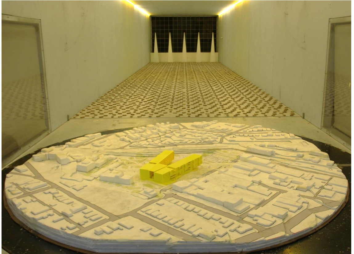
Figure 1b: Photograph of the Wind Tunnel Model (view from the east)
