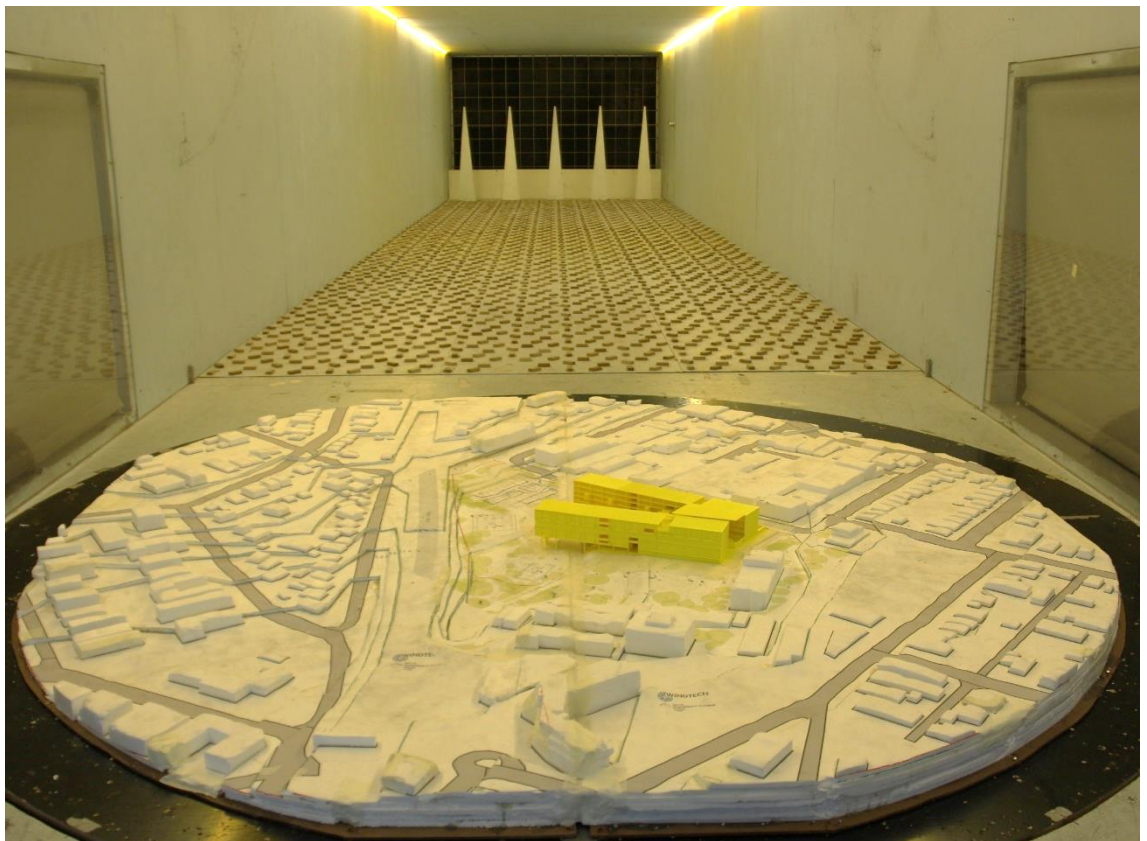
Figure 1a: Photograph of the Wind Tunnel Model (view from the south)
