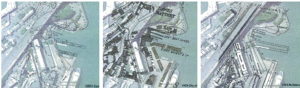
Figure 1.6 Three overlays with 1891, 1903 and 1956 historical overlays showing wharf structures present within the study area. Structures were likely destroyed by construction of the OPT in the late-twentieth century. (Source: Sydney Harbour Foreshore Authority, Campbell's Cove Archaeological Assessment 2012, Appendix B)
