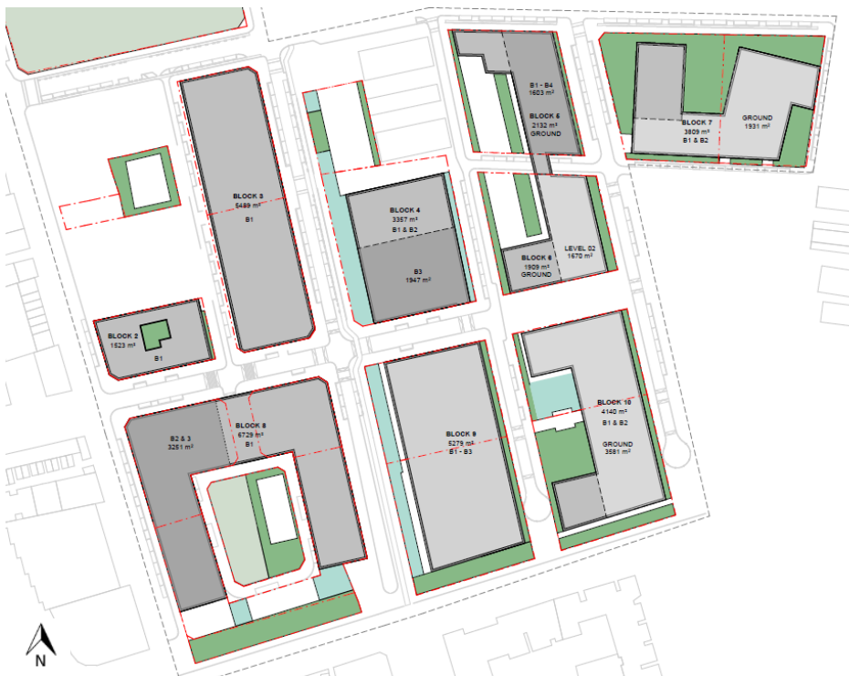
Figure 63 Basement extent plans
