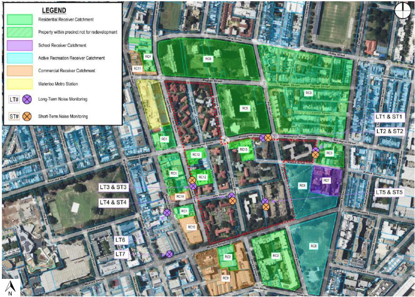
Figure 94 Noise monitoring locations and surrounding sensitive receivers Source: Noise and Vibration Impact Assessment prepared by E-Lab
