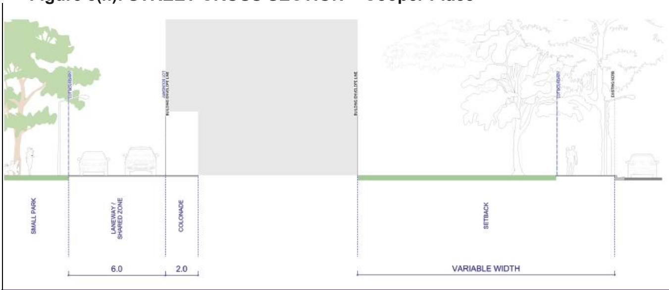
Figure 8(h): STREET CROSS SECTION – Cooper Place
