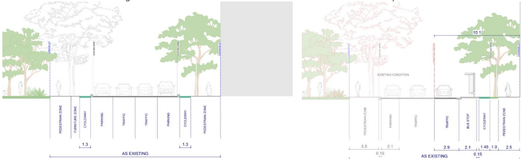
Figure 38: Street Section - Wellington Street (Aspect Studios)
