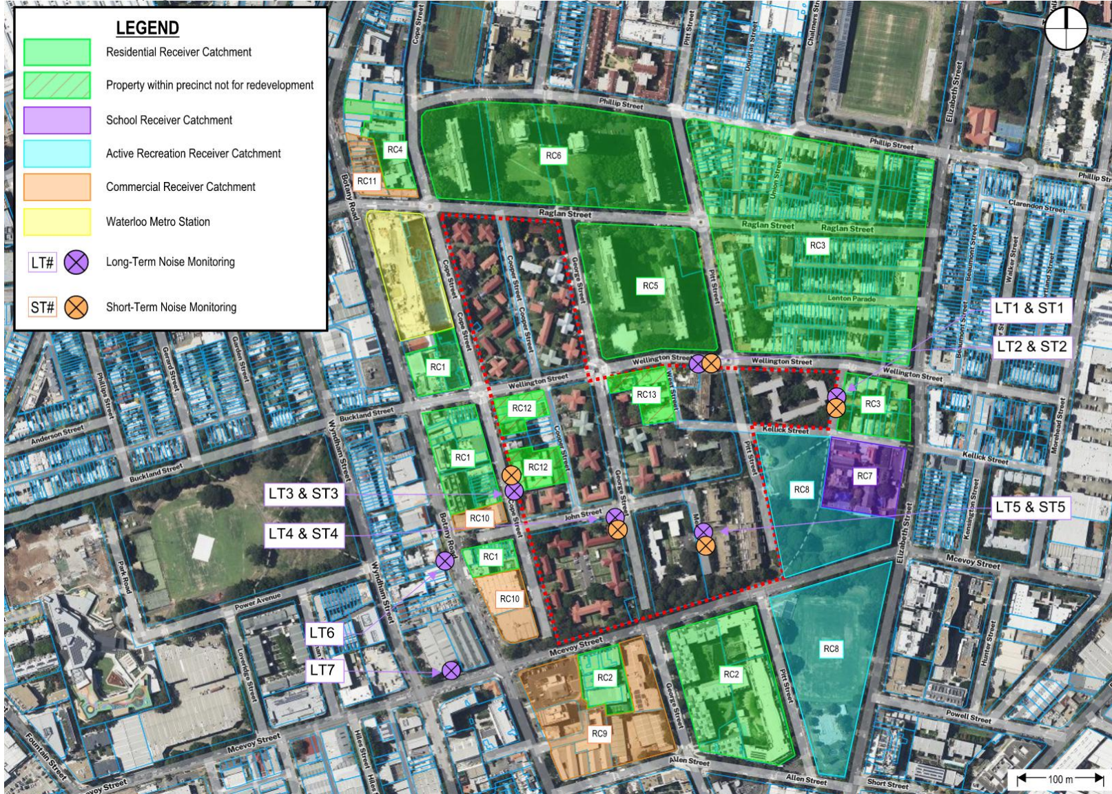
Figure 3: Acoustic site plan identifying the surrounding noise-sensitive receivers and noise monitoring locations
