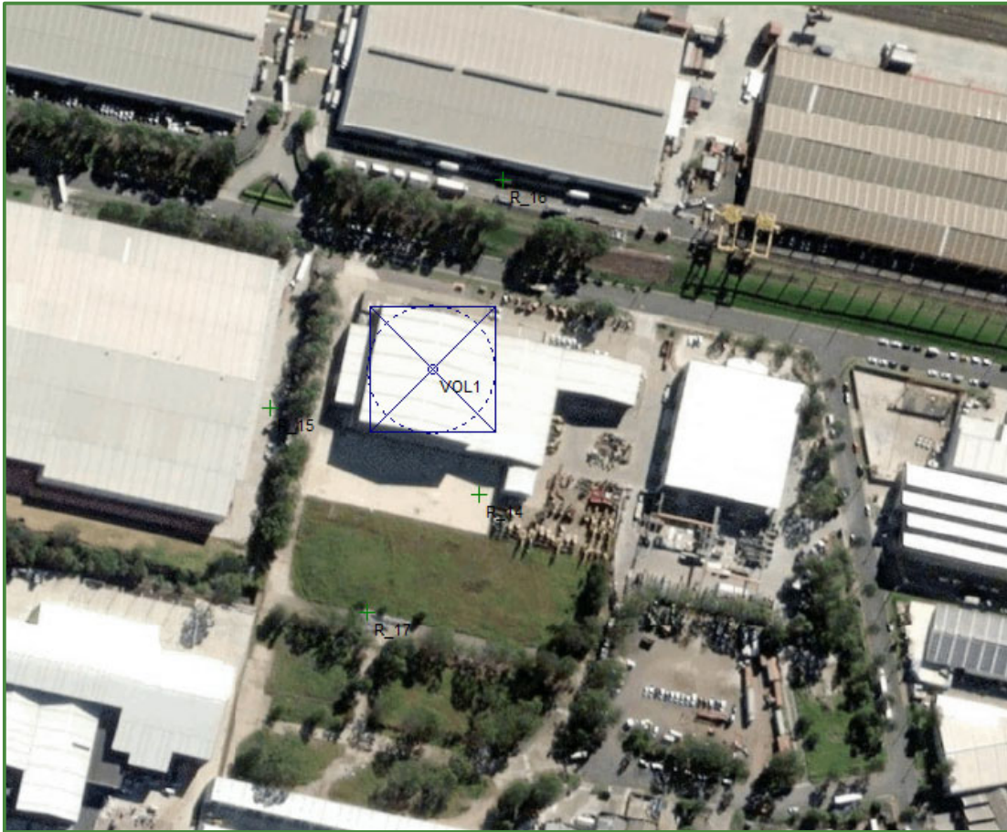
Figure 6-1: Arrangement of Modelled Volume Source
