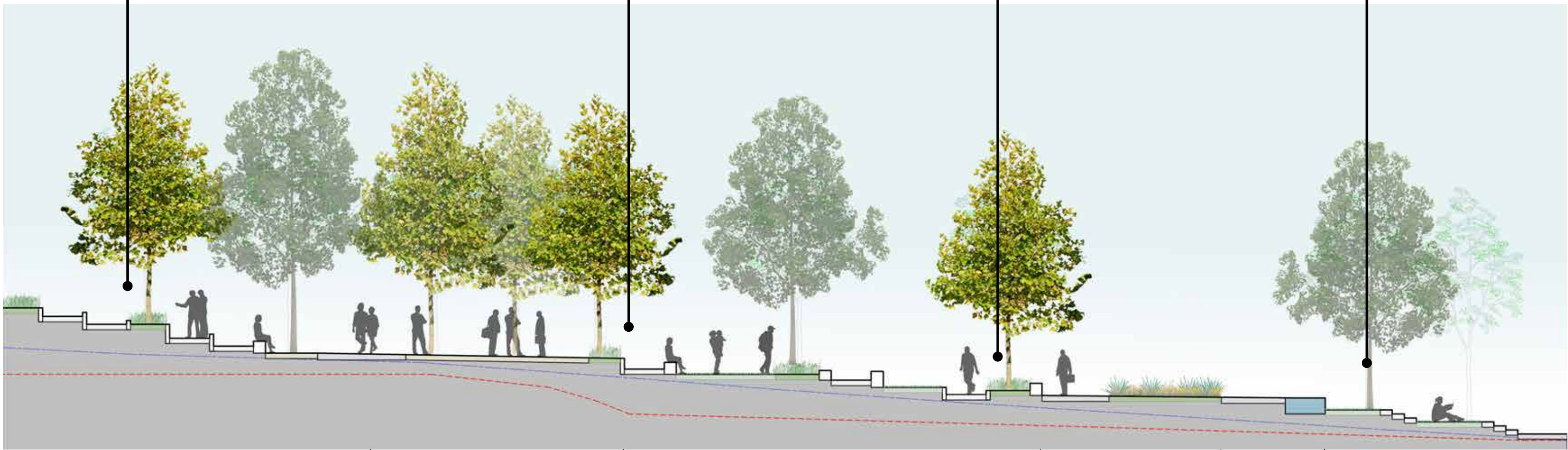
Terraced landscape with 1:21 pedestrian ramps Mixed grove planting within turf Terraced landscape with 1:21 pedestrian ramps Planted landscape terrace Linear water feature Inhabitable seating edges
