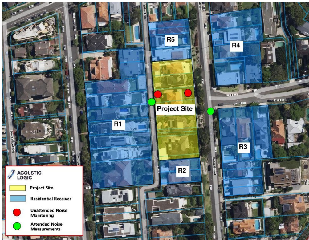
Figure 30 Extract from Acoustic Assessment showing Sensitive Receivers
