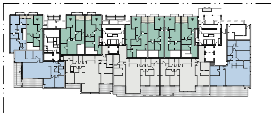
PLAN Level 02 1:750 Note: * denotes two storey terraces which only count once for cross ventilation
