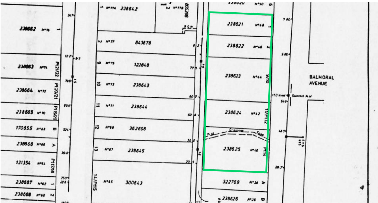
Figure 12 – Sydney Water plan of the subject area, 1982, showing easement for drainage through No. 40.
