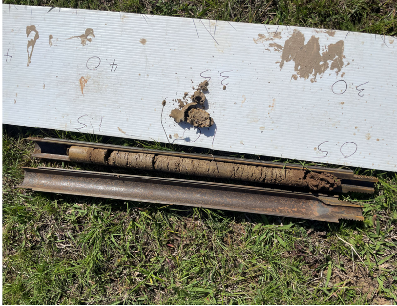
Photo 5 - Typical cutting from Standard Penetration Test
