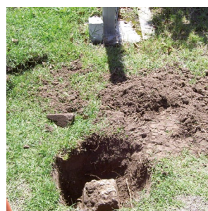
Concrete Block references boundary corner (peg)
