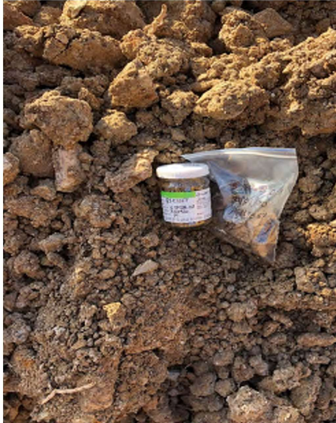
Photo 3. Sample of reworked natural CLAY with sand obtained from STP02
