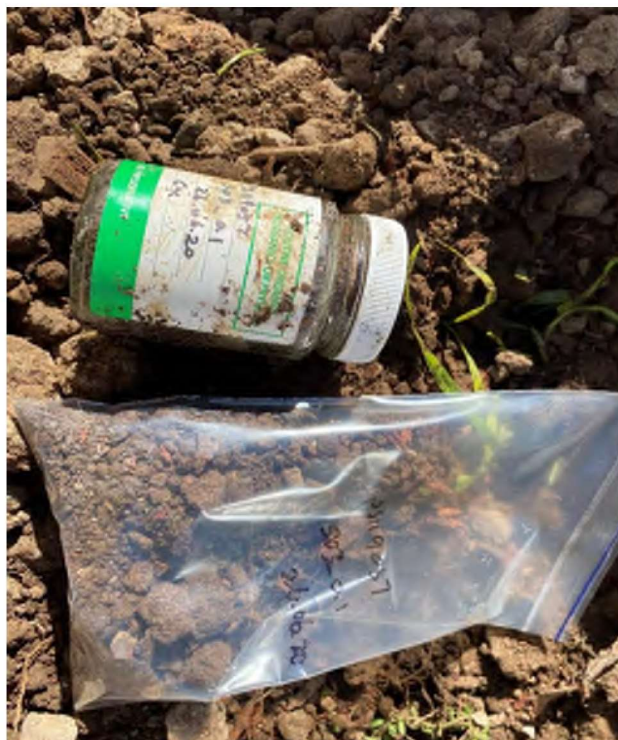
Photo 4. Example of sandy gravelly material observed in S03_0.1.
