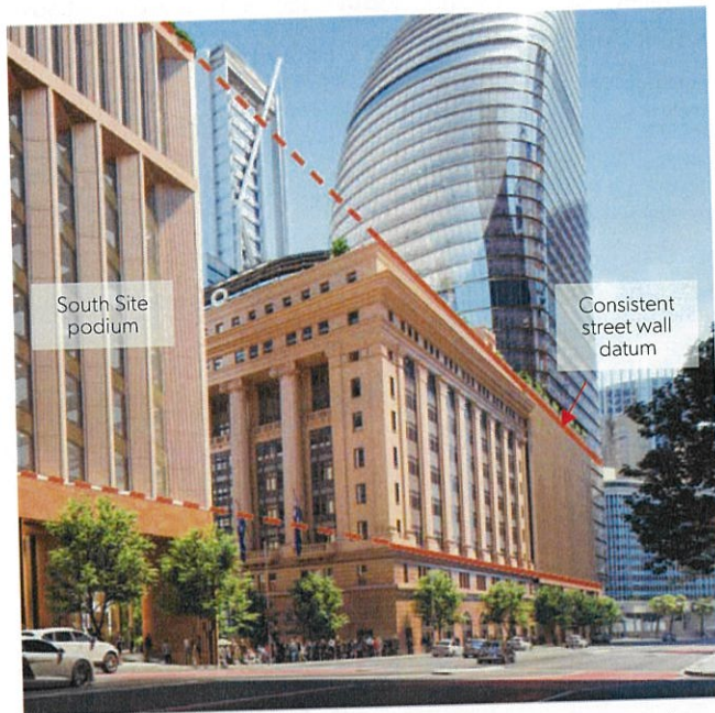
Figure 20 | Photomontage of 50 Martin Place with the height datum of its parapet. The proposed podium as defined by the southern terrace also matches the height of the proposed South Site podium (Source: Applicant's RtS)
