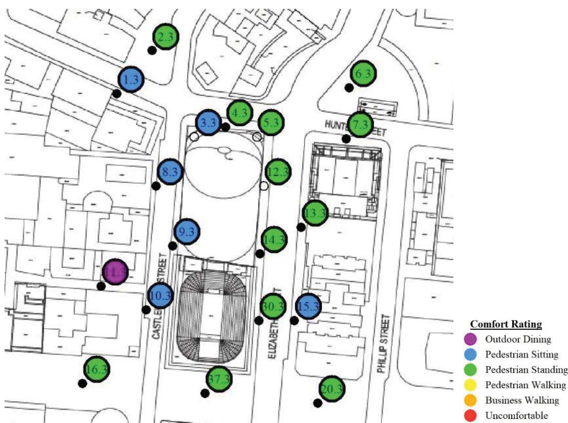
Figure 89 Locations and results of the wind tunnel testing (proposed detailed design)
