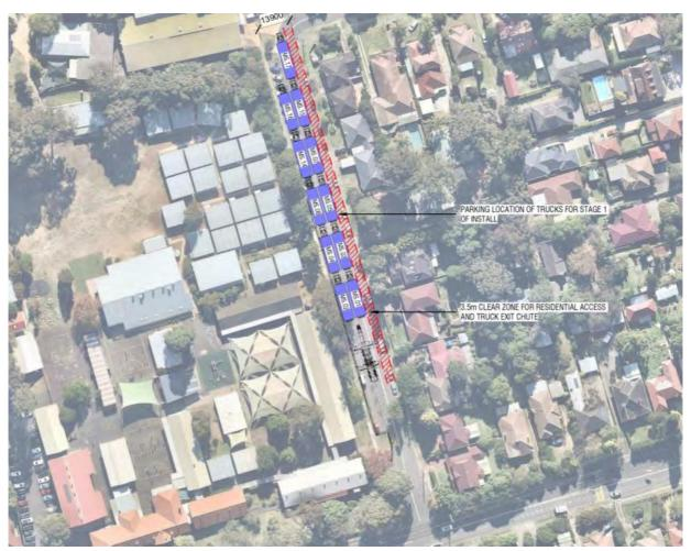
Figure 13: Indicative diagram of Stage 1 Modules on Ward Street (Source: Modscape; Detailed Design Buildability Workshop)
