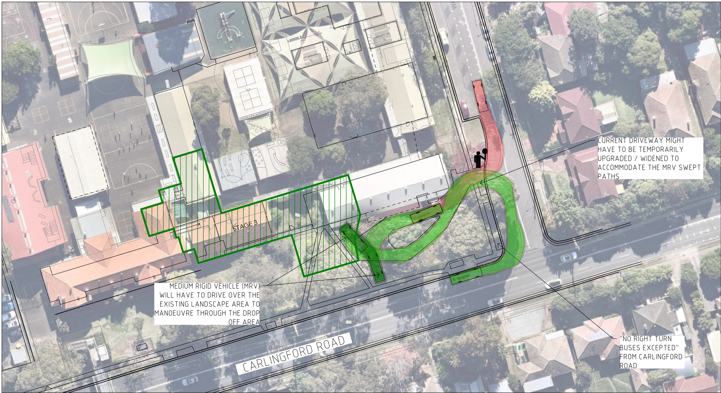
MEDIUM RIGID VEHICLE (8.8m MRV) SWEEP PATHS
