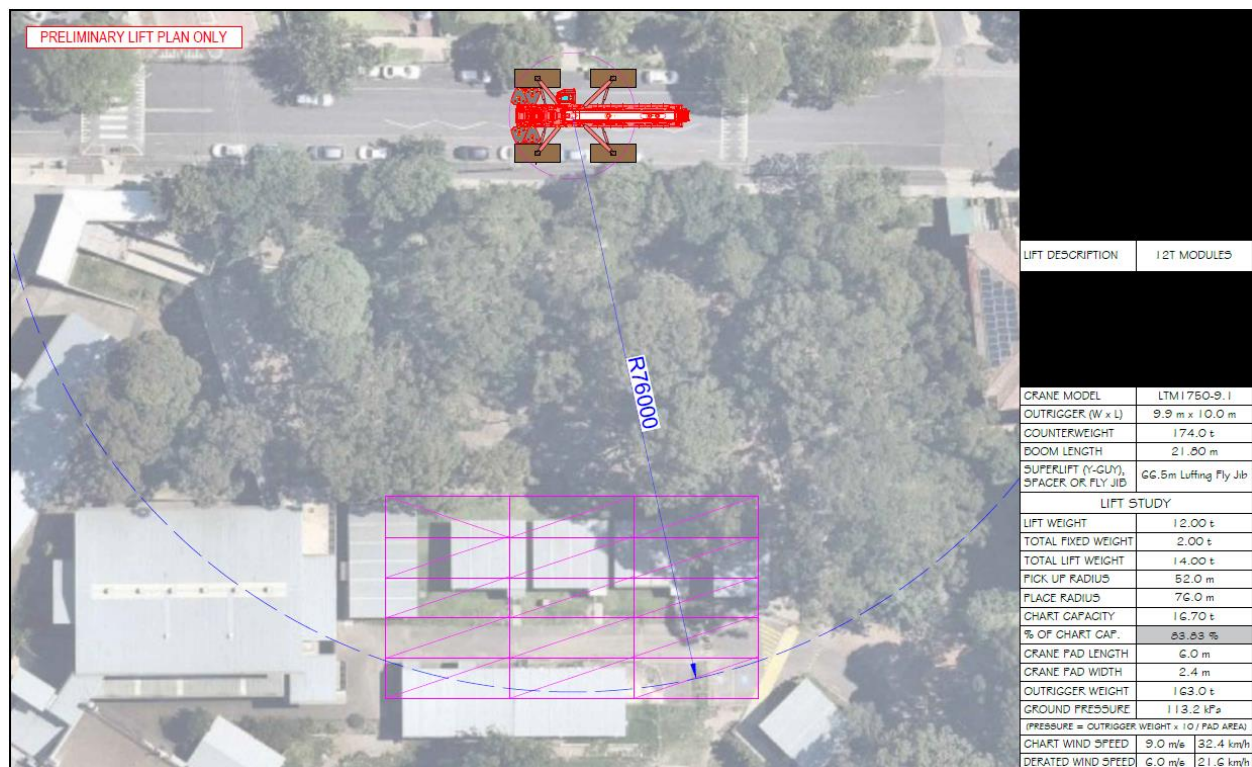
Figure 7-3 Example plan for crane location on street
