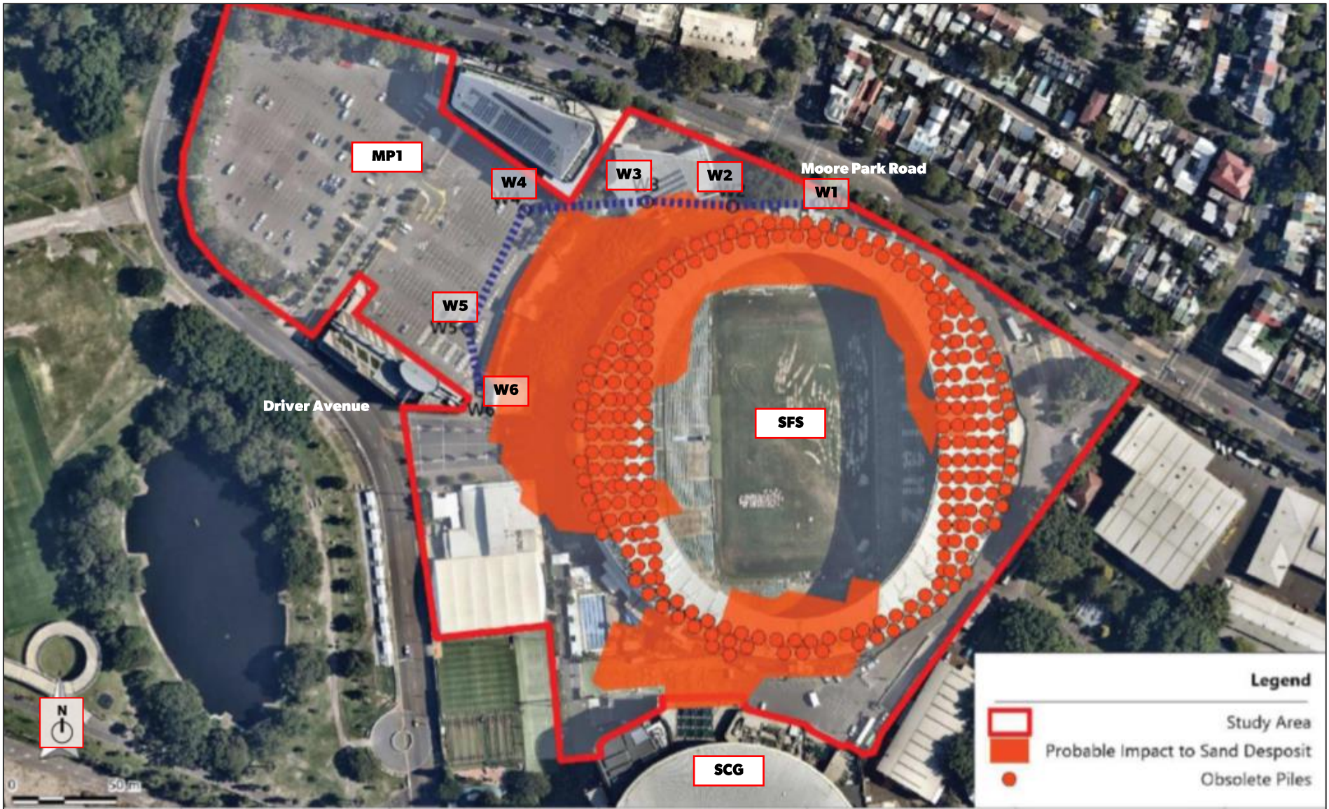
Figure 8 | Below ground works overlaid on the indicative natural sand profile impact zones (Source: Applicant's Modification Report)
