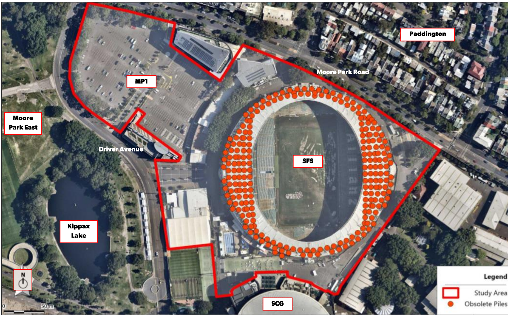
Figure 3 | Location of the former SFS in the local context and the piles that are proposed to be removed (Source: Applicant’s Modification Report)
