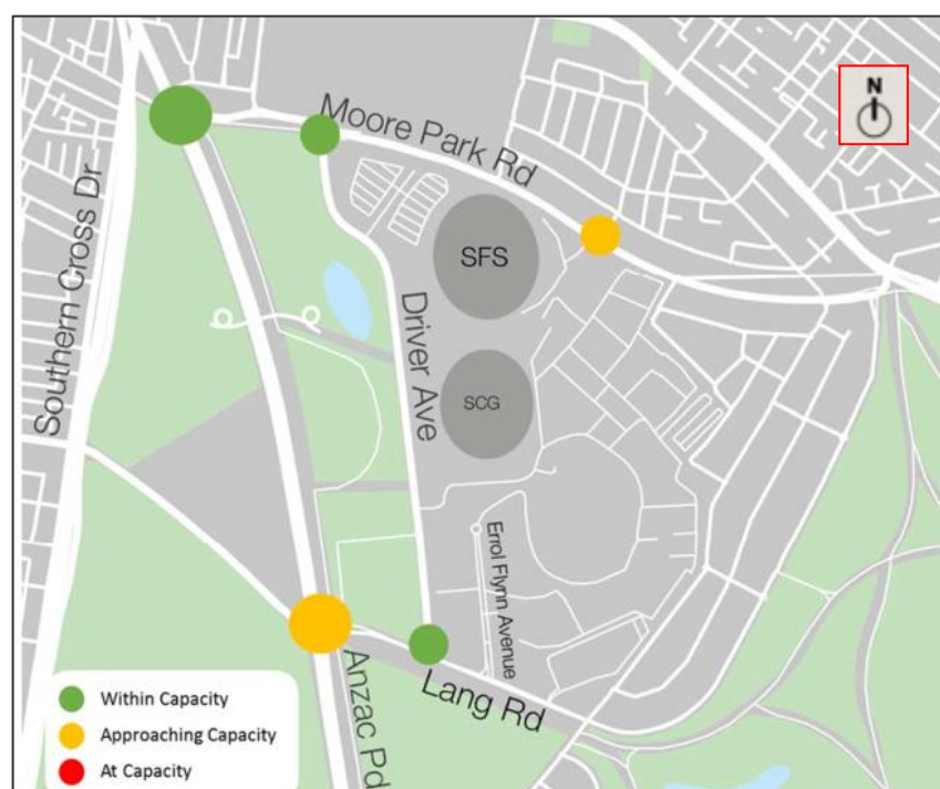
Figure 34 | Intersection locations and existing pre-event performance (Source: Applicant's RtS)
