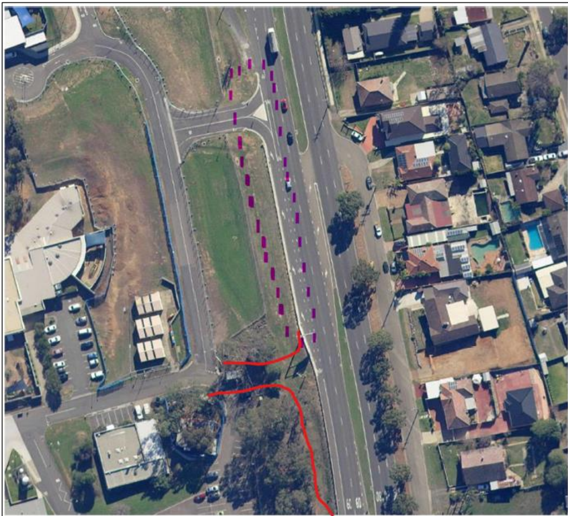
Figure 2 | Redundant deceleration lane and entry (within purple dotted lines) and previously approved new hospital access in red (Source: Enstruct Traffic Design Report)
