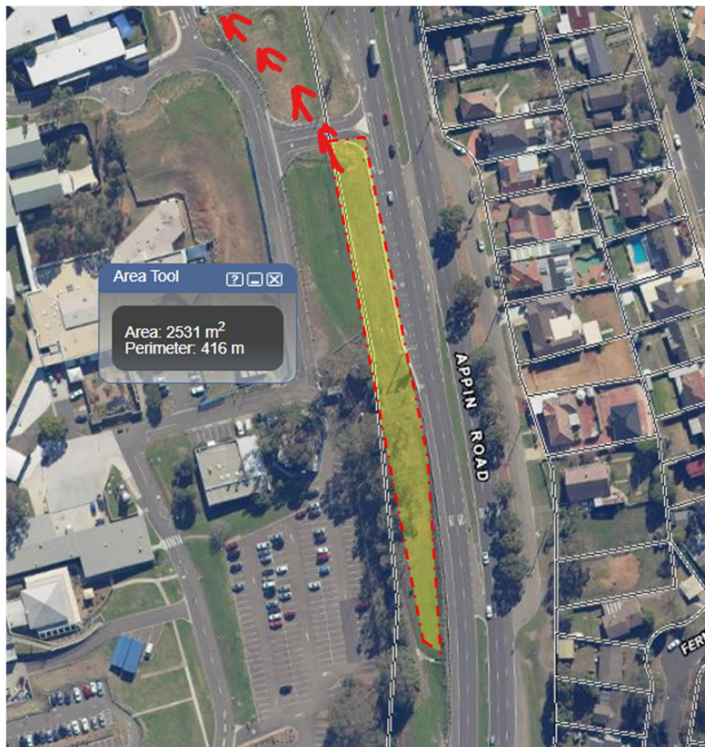
Figure 4 – Road Reserve Draining into the Hospital
