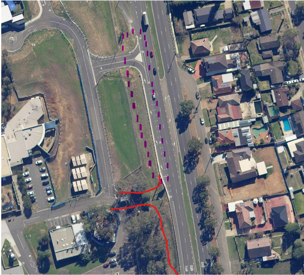
Figure 1 - Existing Deceleration Lane and Proposed Access
