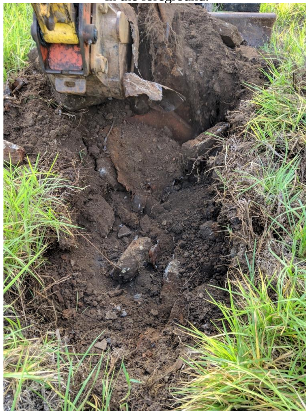
Photo No 12 – Test Pit No 4 ; Rubbish fill including metal, concrete and bricks encountered in the backfilled depression area (Site Feature G)
