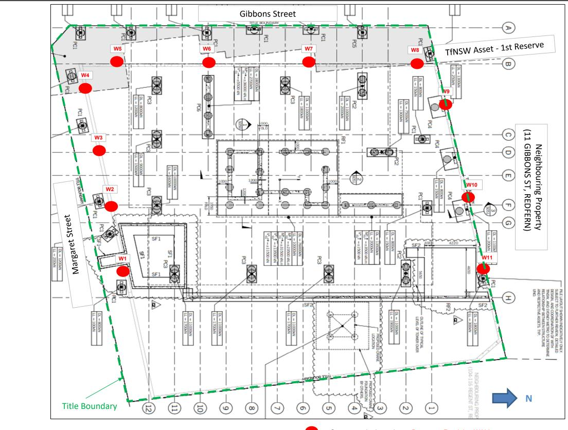
Survey monitoring point on **Basement Retaining WALL**
