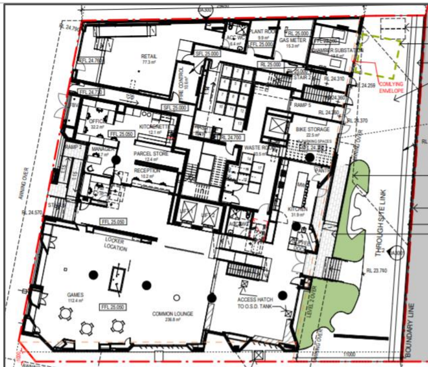
Figure 5 | Proposed ground floor plan. Minor amendments to the size of rooms are shown. (Source: Submitted architectural plans)
