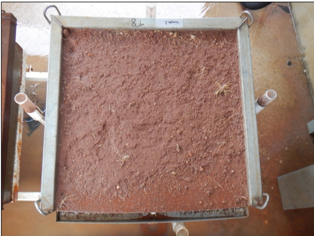
Photograph B 2. Chromosol/Sodosol Topsoil test plot after receiving simulated rain at 100–125 mm/hr.
