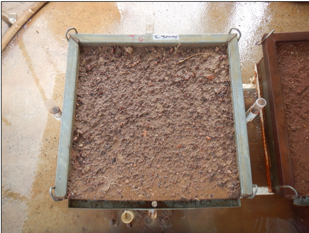
Photograph B 6. Gilgai Topsoil test plot after receiving simulated rain at ~100–125 mm/hr.
