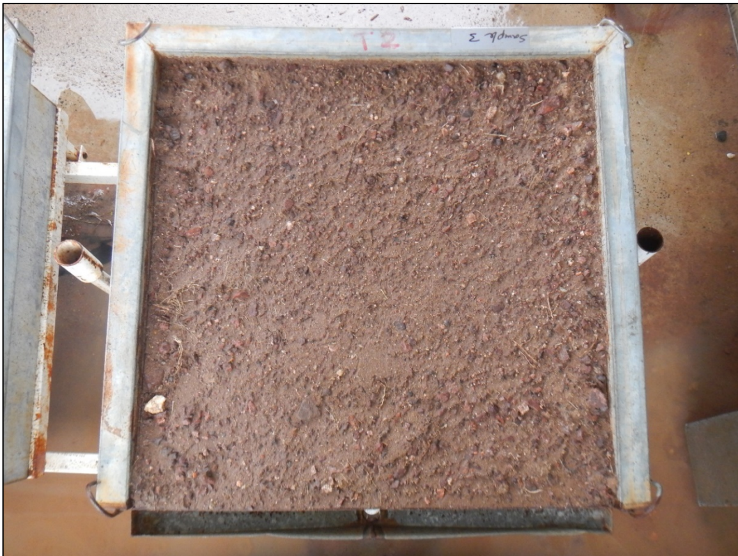
Photograph B 4. Chromosol Subsoil test plot after receiving simulated rain at ~100–125 mm/hr.
