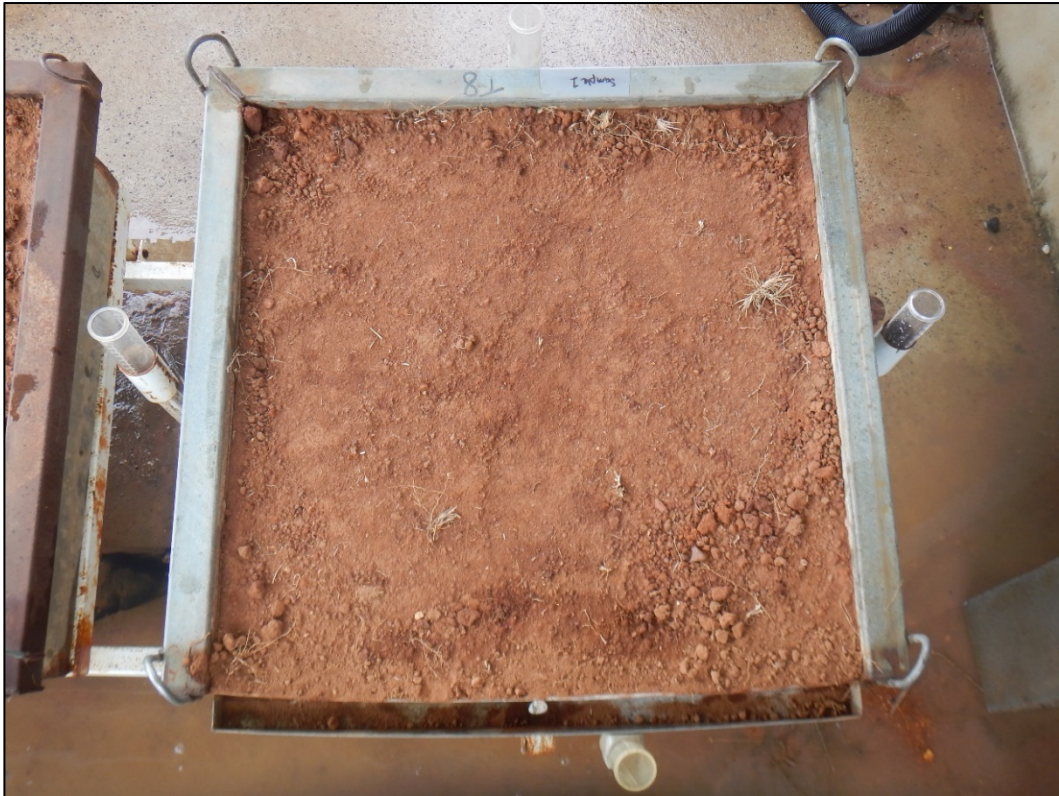
Photograph B 1. Chromosol/Sodosol Topsoil test plot prior to rainfall simulation.
