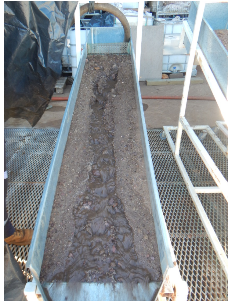
Photograph B 12. Gilgai Topsoil plot tested to failure with overland flows.
