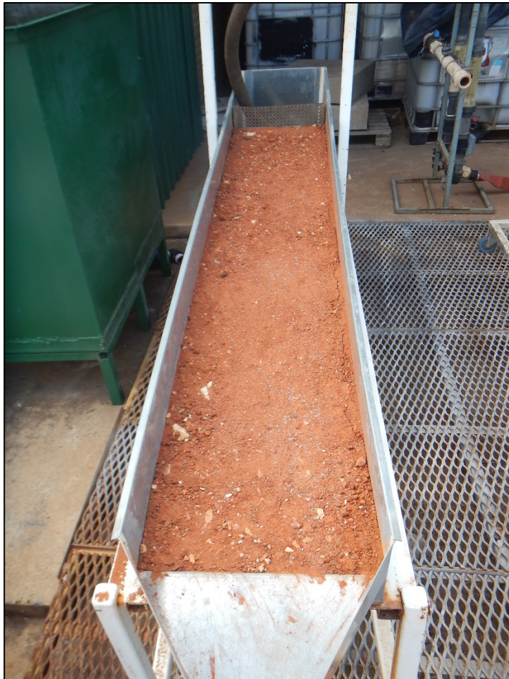
Photograph B 7. Chromosol/Sodosol Topsoil plot prior to being subjected to overland flows.
