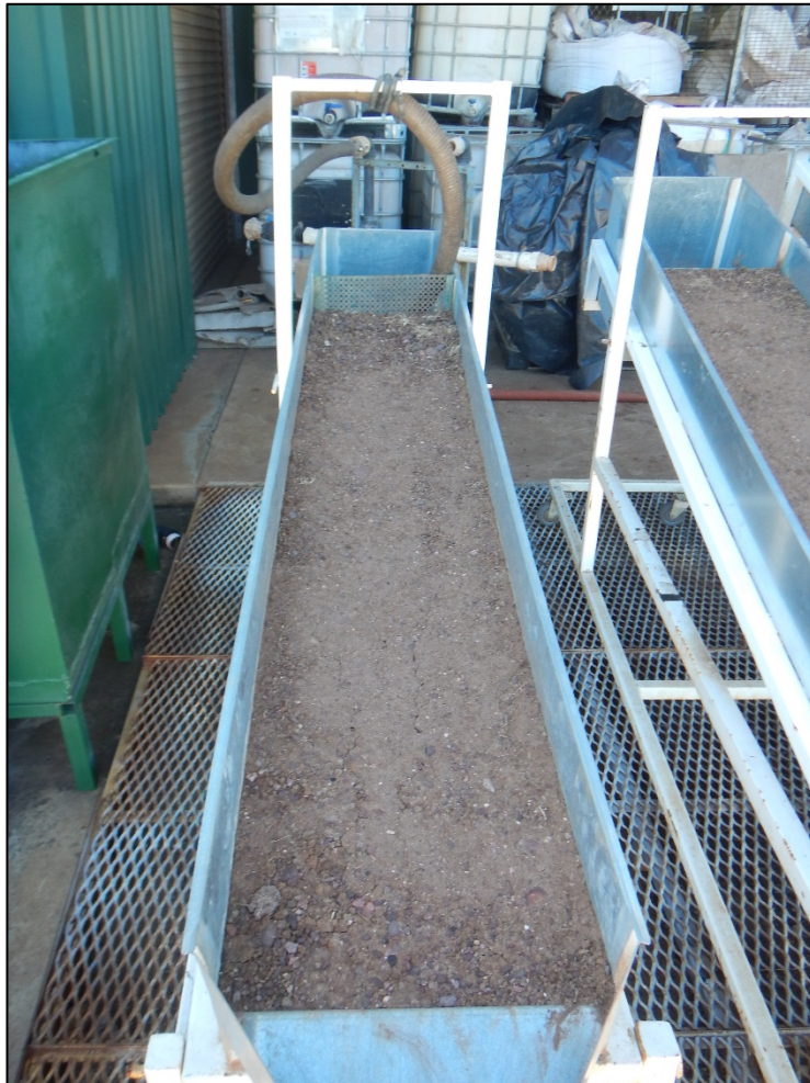
Photograph B 11. Gilgai Topsoil plot prior to being subjected to overland flows.
