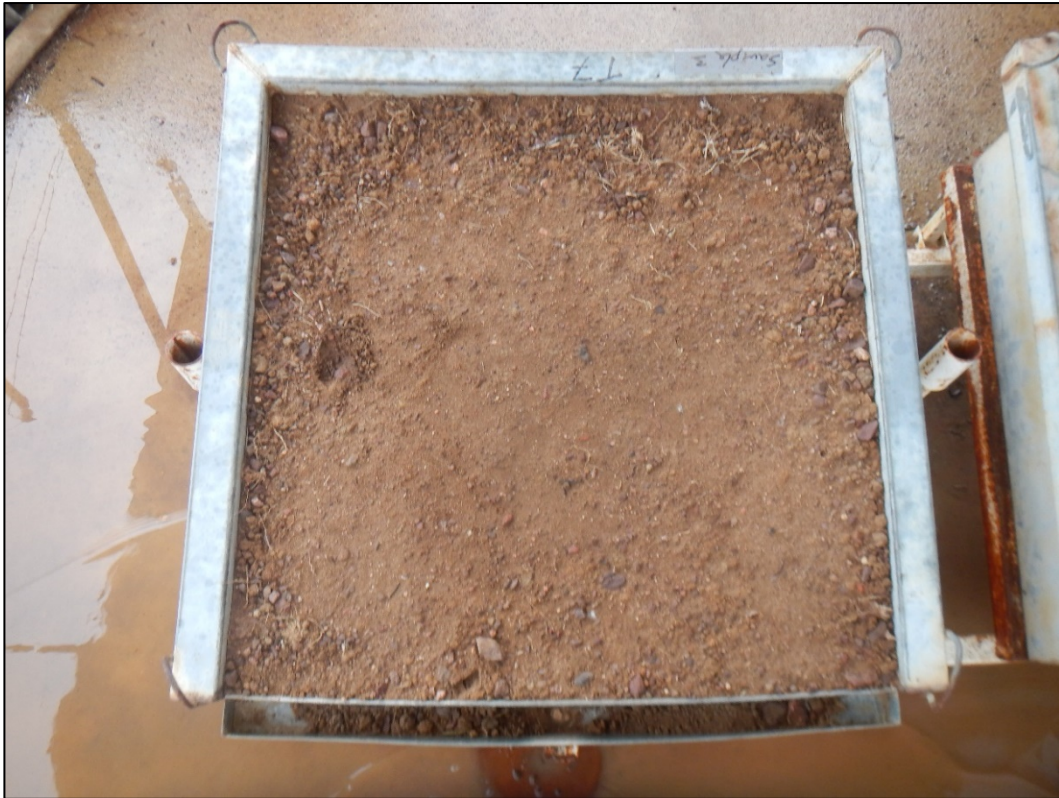
Photograph B 3. Chromosol Subsoil test plot prior to rainfall simulation.
