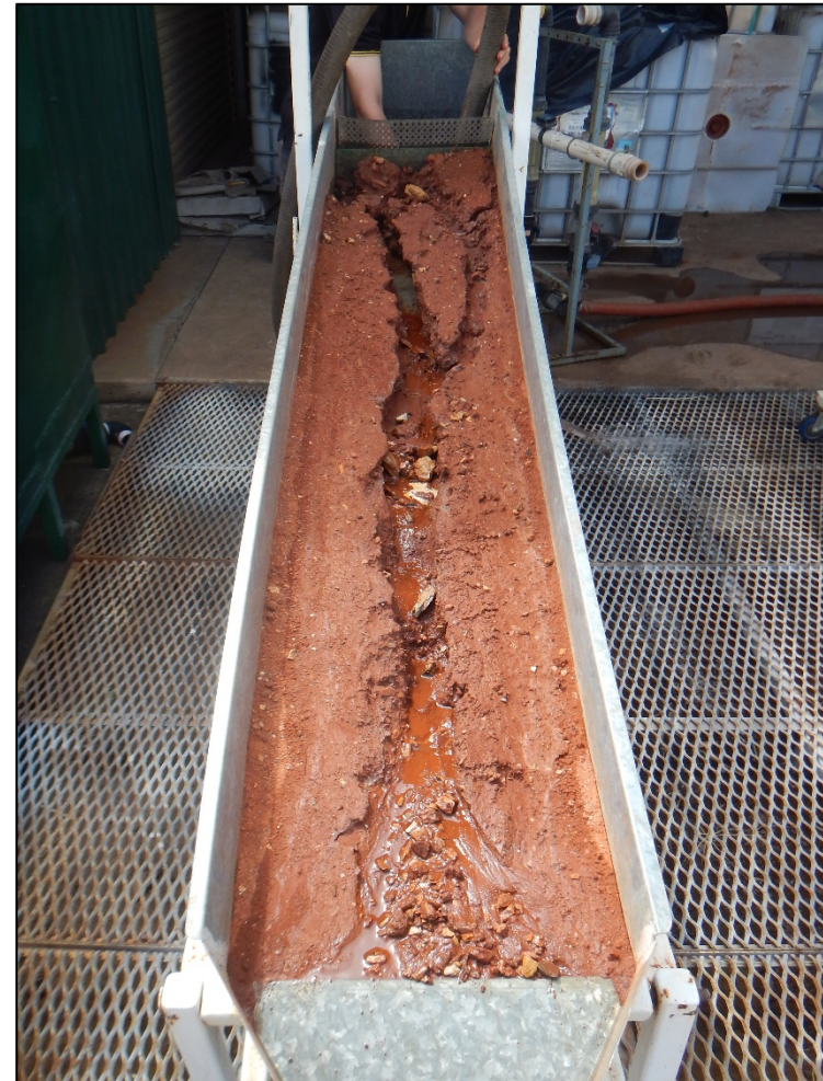
Photograph B 8. Chromosol/Sodosol Topsoil plot tested to failure with overland flows.
