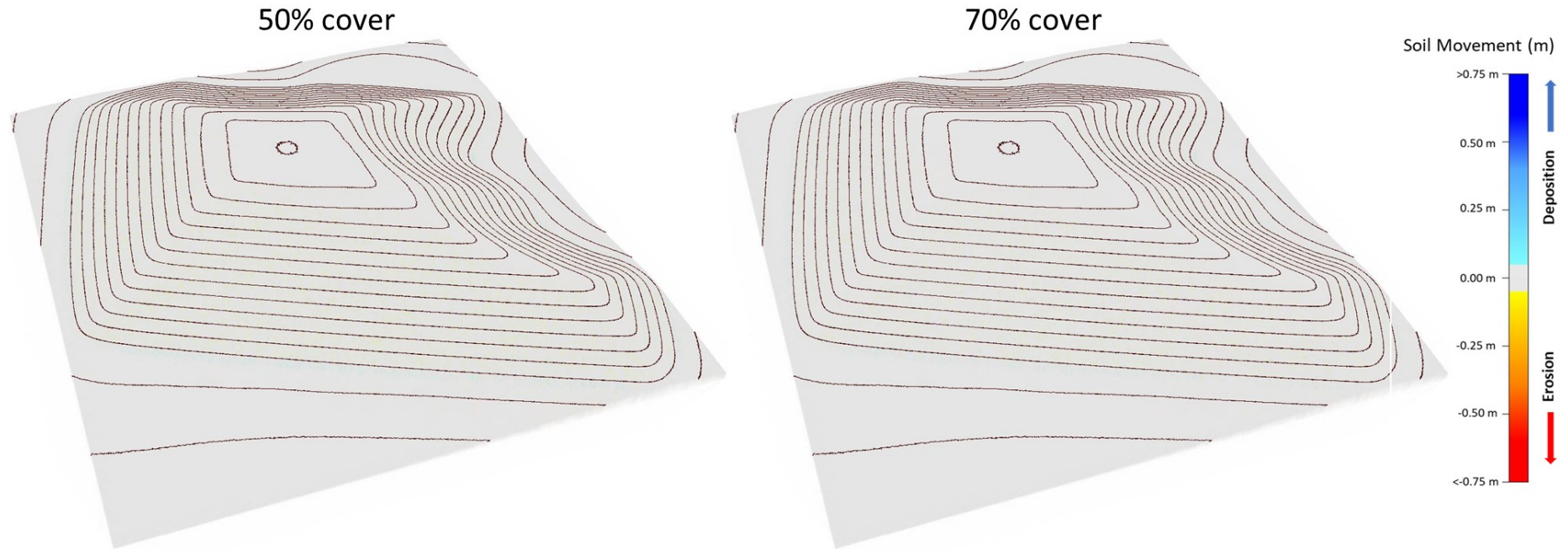
Figure C 1. Landform evolution model after 10 years of the SAR WRE covered with CH/SO Topsoil cover 0.3 m thick and vegetation cover of 50 % and 70 %. There are negligible areas where appreciable erosion or deposition is predicted to occur.
