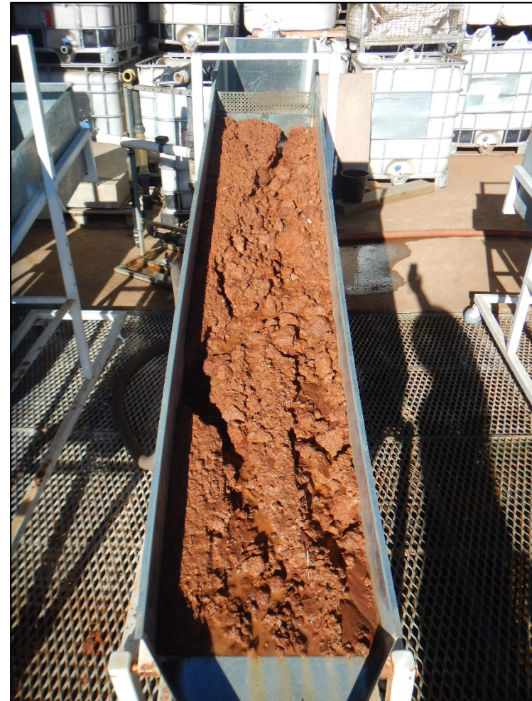
Photograph B 10. Chromosol Subsoil plot tested to failure with overland flows.
