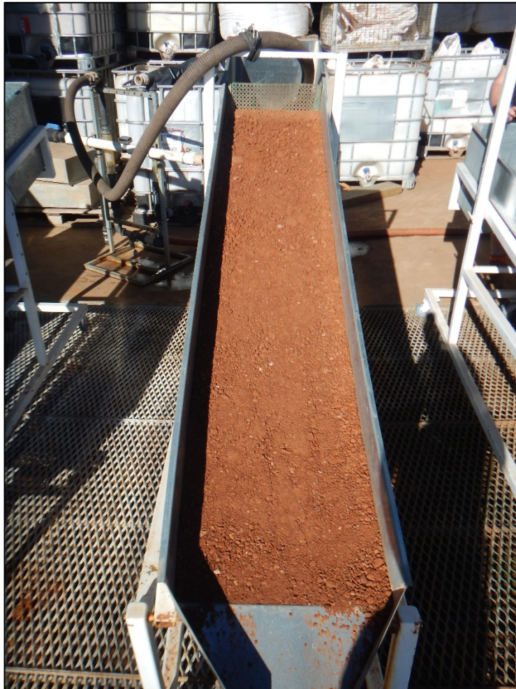
Photograph B 9. Chromosol Subsoil plot prior to being subjected to overland flows.
