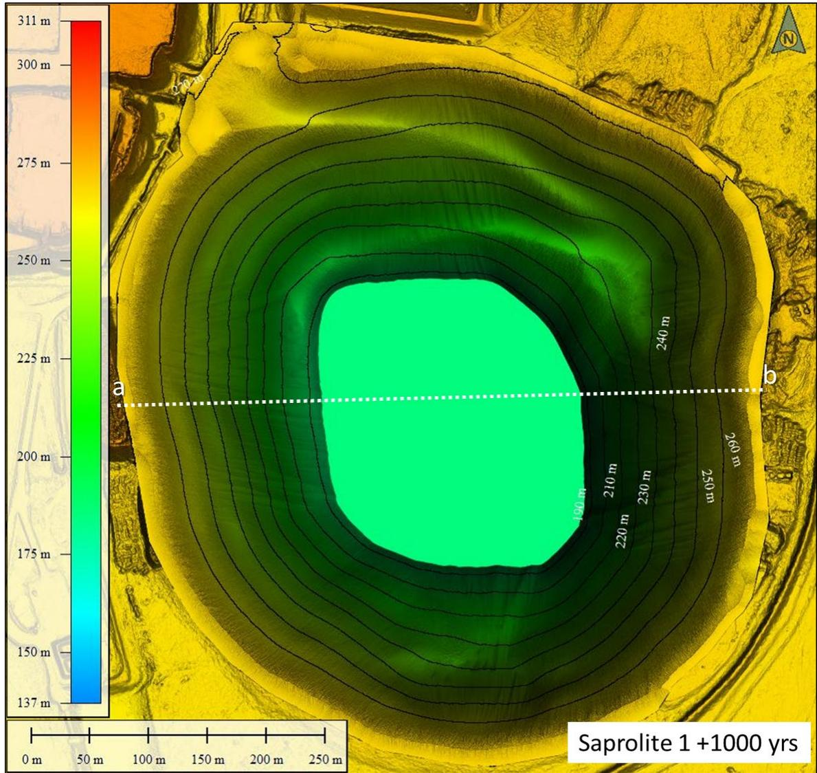
**Figure B 11:** Landform evolution model output after 1,000 years of the Wyoming 1 Pit with a Saprolite 1 surface in a bare (unvegetated) condition.
