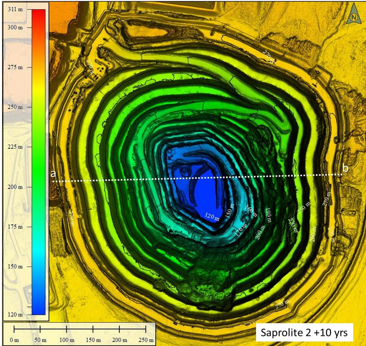
**Figure B 13:** Landform evolution model output after 10 years of the Wyoming 1 Pit with a Saprolite 2 surface in a bare (unvegetated) condition.
