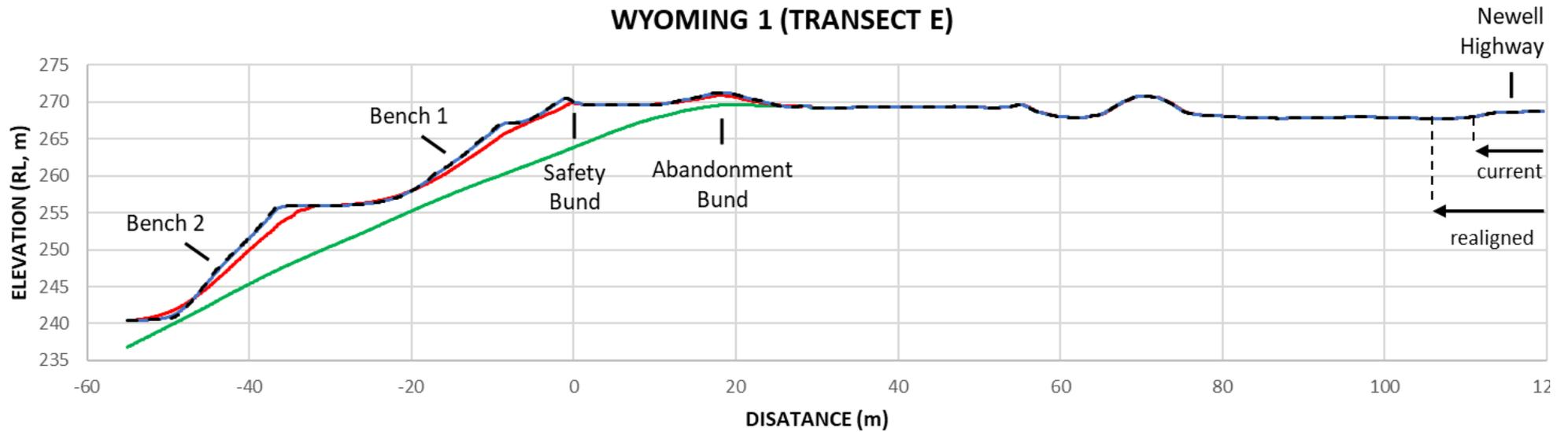
Figure 6: Cross-sections Transect N and Transect E of the residual Wyoming 1 Open Cut at timescales of 0, 10, 100, and 1,000 years.
