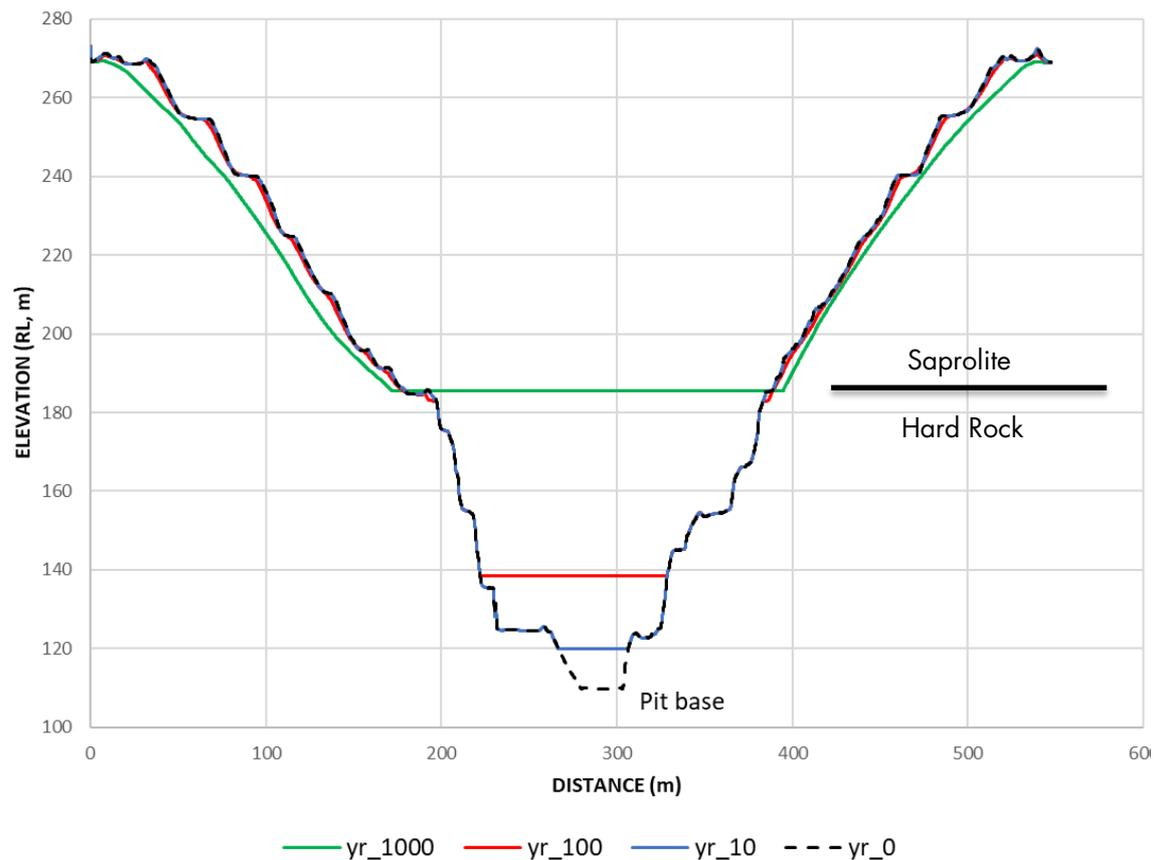
**Figure 10:** Conceptual representation of deposition levels of eroded sediment into Wyoming 1 Open Cut at time intervals of 10, 100, and 1,000 years.
