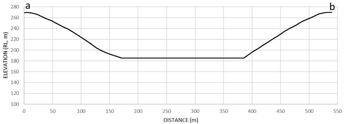
**Figure B 6:** Cross section of the transect in Figure B 5. Note the interface of the batters and berms is no longer detectable due to erosion of the pit wall.
