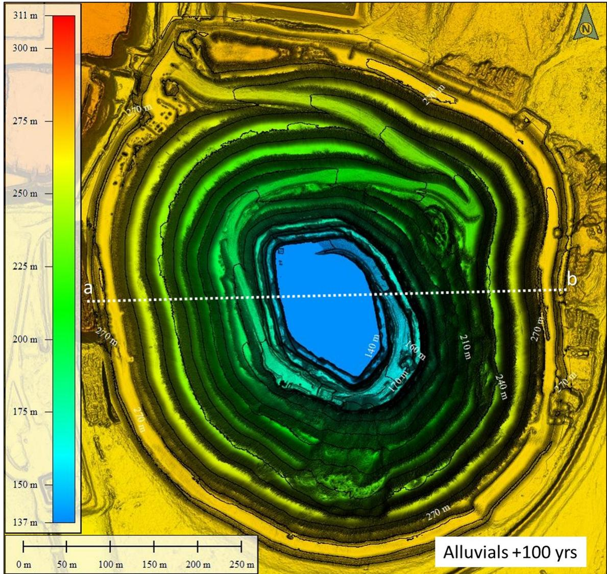
**Figure B 3:** Landform evolution model output after 100 years at the Wyoming 1 Pit with an Alluvial surface in a bare (unvegetated) condition.
