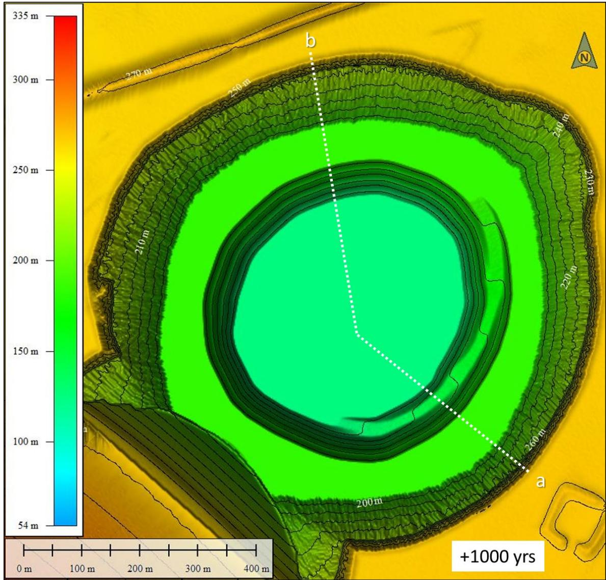
**Figure B 23:** Landform evolution model output after 1,000 years of the SAR North Pit with a Sapolite 1 surface in a bare (unvegetated) condition.
