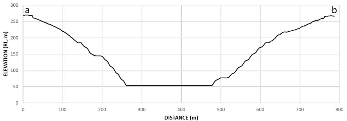
**Figure B 22:** Cross section of the transect in Figure B 21. Note the interface of the batters and berms has smoothed relative to the 10 year simulation due to erosion at the crest of the berms and deposition at the toe of the batters.
