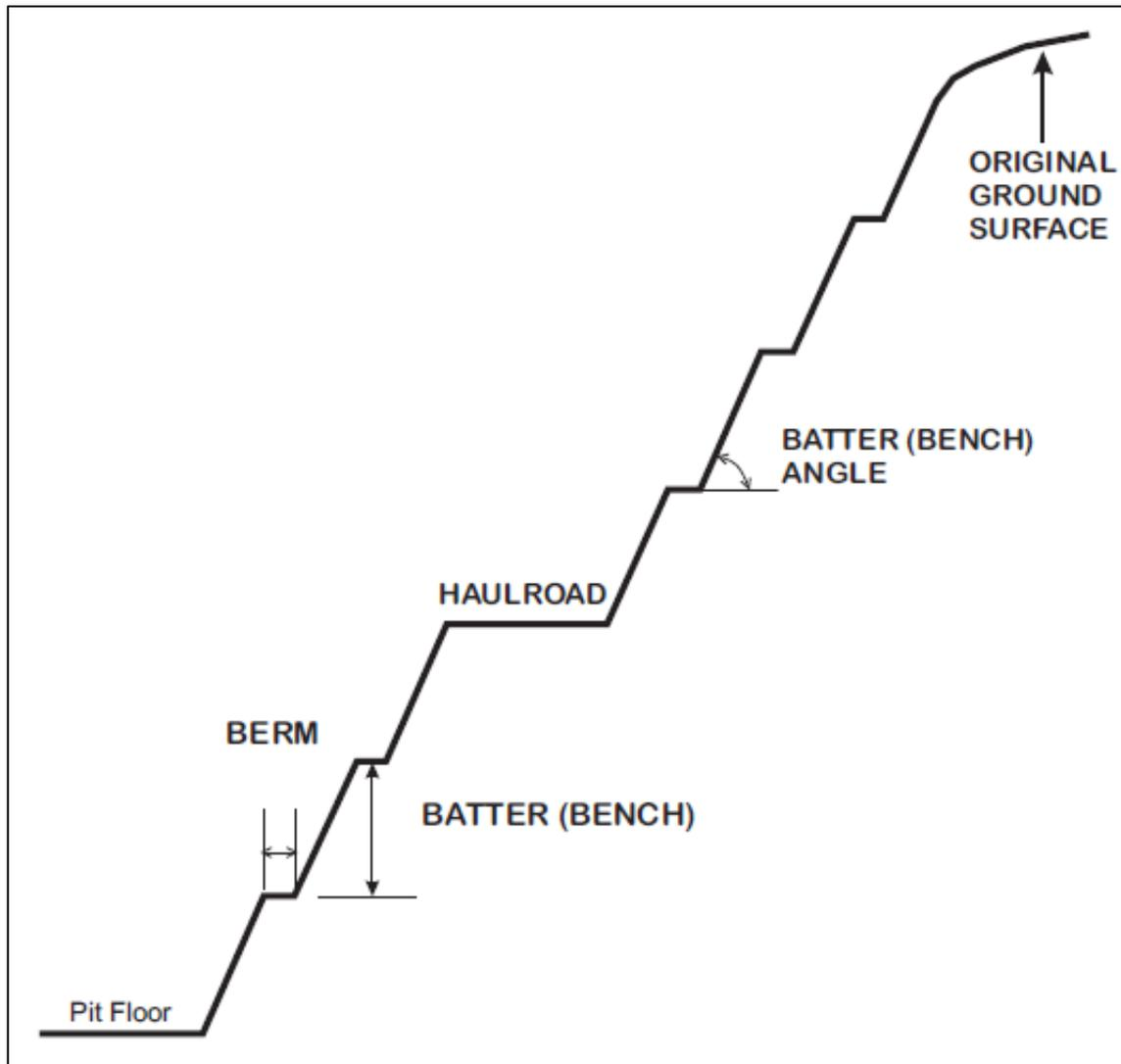
Figure 2. Generalised cross-section of the pit (Mining One, 2010).
