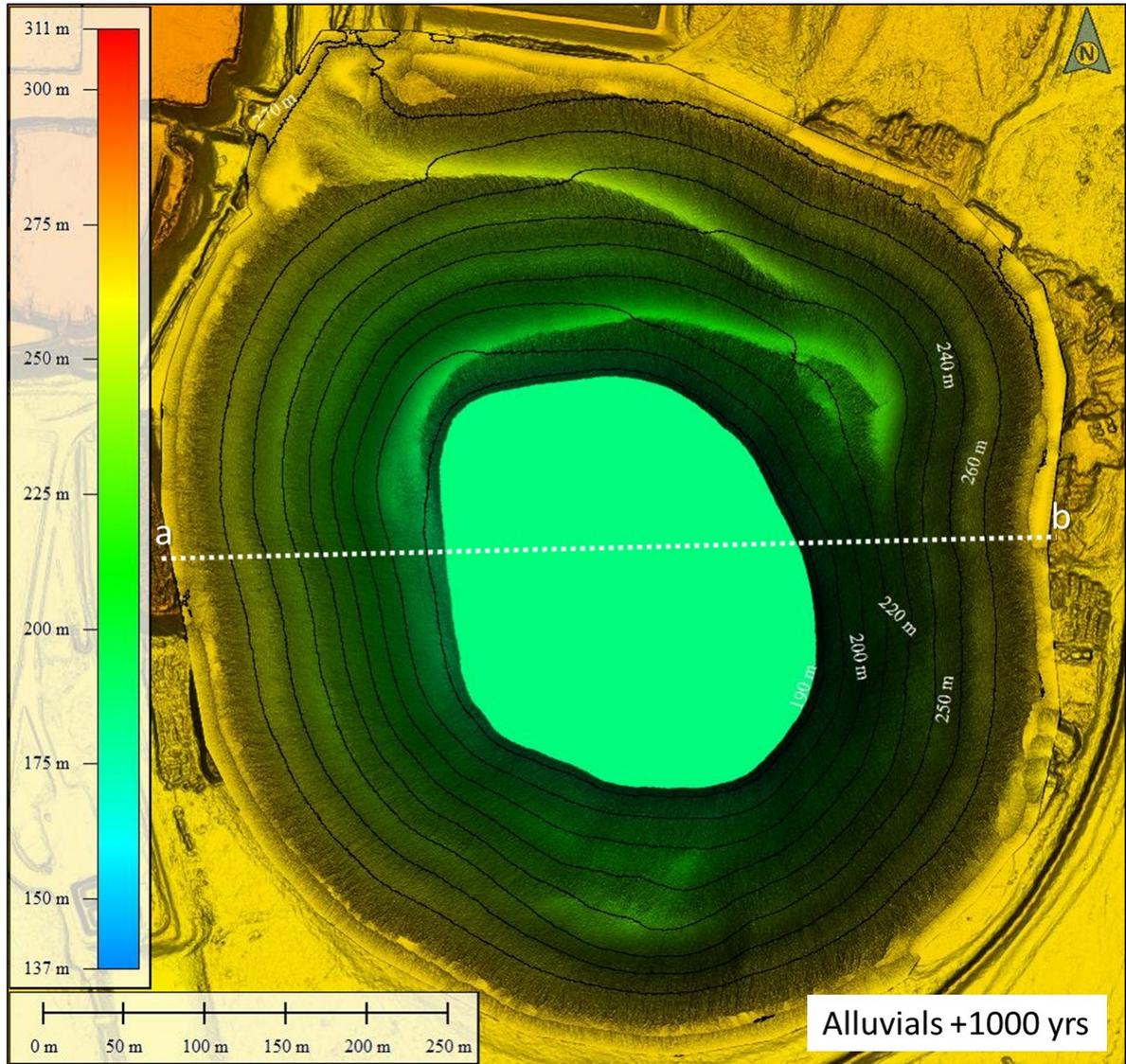
**Figure B 5:** Landform evolution model output after 1000 years at the Wyoming 1 Pit with an Alluvial surface in a bare (unvegetated) condition.
