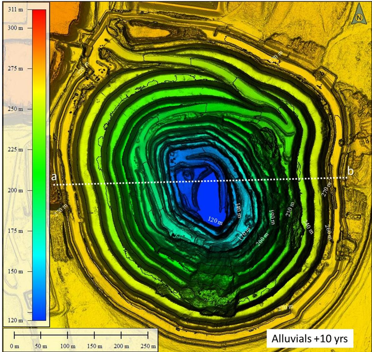
**Figure B 1:** Landform evolution model output after 10 years at the Wyoming 1 Pit with an Alluvial surface in a bare (unvegetated) condition.
