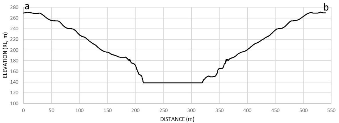
Figure B 8: Cross section of the transect in Figure B 7. Note the interface of the batters and berms is distinct and similar to present day conditions.
