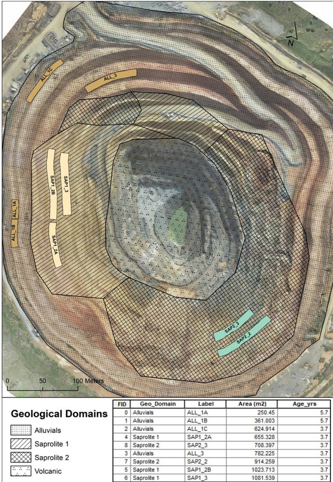
Figure A 3. Calibration areas within Wyoming 1 Pit and conceptual model of the lithologies of interest.
