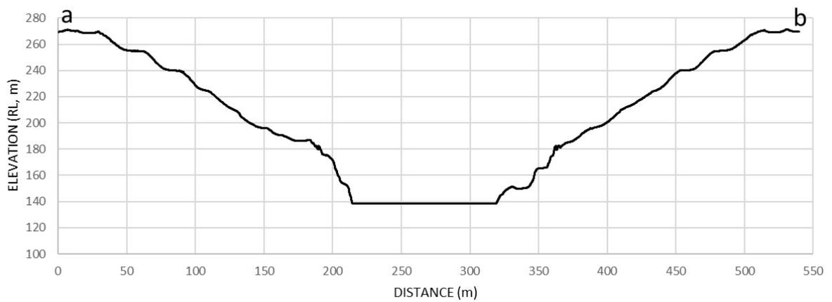
**Figure B 4:** Cross section of the transect in Figure B 3. Note the interface of the batters and berms has smoothed relative to present day conditions due to erosion at the crest of the berm and deposition at the toe of the batter.
