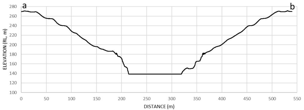
**Figure B 16:** Cross section of the transect in Figure B 15. Note the interface of the batters and berms has smoothed relative to present day conditions due to erosion at the crest of the berm and deposition at the toe of the batter.
