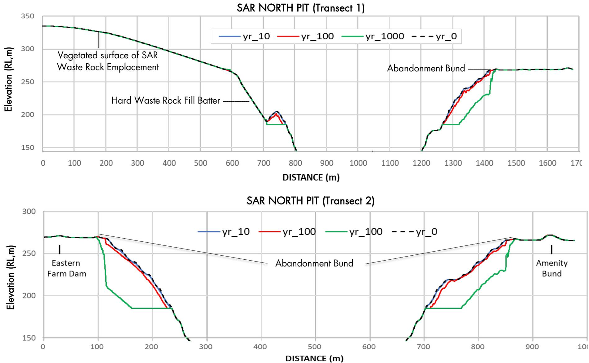
Figure 9: Cross-sections Transect 1 and Transect 2 of the residual SAR North Pit at timescales of 0, 10, 100, and 1,000 years.
