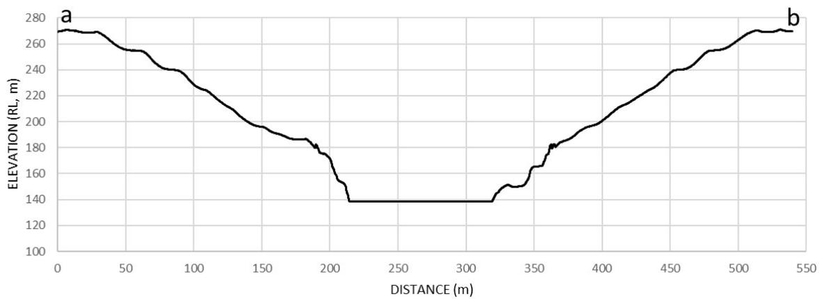
Figure B 10: Cross section of the transect in Figure B 9. Note the interface of the batters and berms has smoothed relative to present day conditions due to erosion at the crest of the berm and deposition at the toe of the batter.
