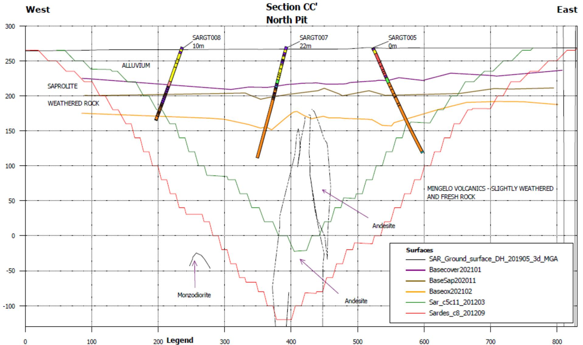
Figure A 5: Cross-section of lithologies of the SAR North Pit at Transect DD displayed in Figure A4 (WSP, 2021).
