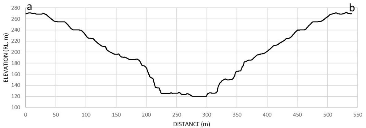
**Figure B 2:** Cross section of the transect in Figure B 1. Note the interface of the batters and berms is distinct and similar to present day conditions.
