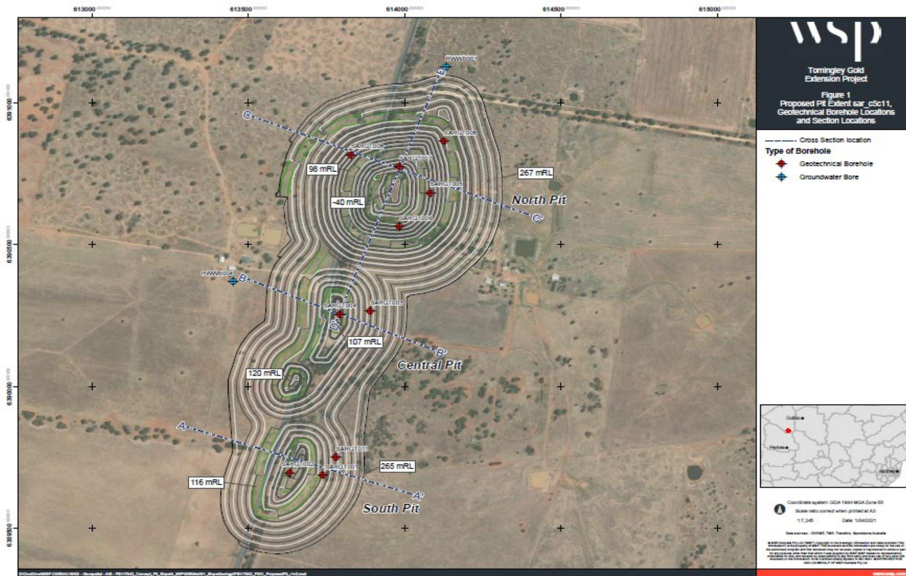
Figure A 4: Proposed extent of the North, Central, and South Pits of the SAR Open Cut. Locations of geotechnical boreholes and cross sections shown (WSP, 2021).
