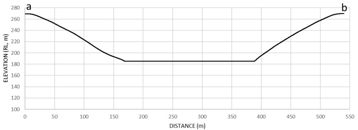
**Figure B 12:** Cross section of the transect in Figure B 11. Note the interface of the batters and berms is no longer detectable due to erosion of the pit wall.
