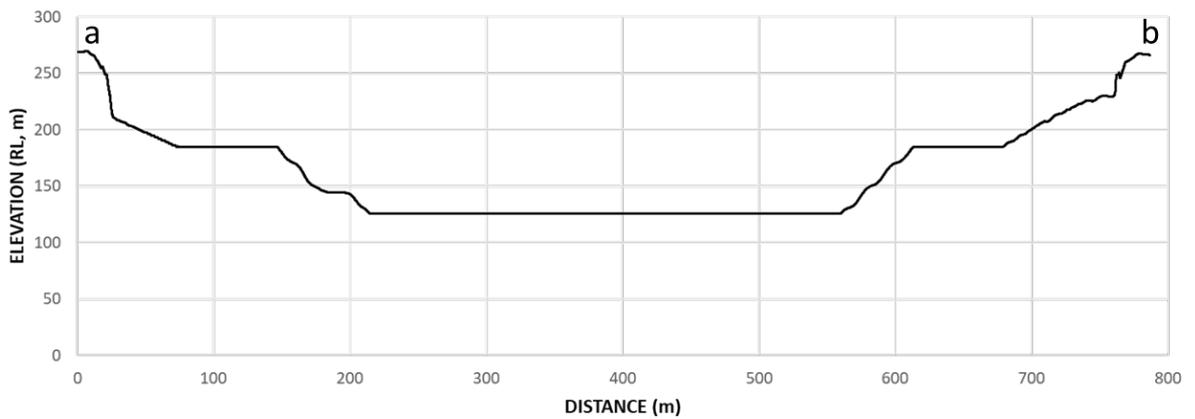
**Figure B 24:** Cross section of the transect in Figure B 23. Note the interface of the batters and berms is no longer detectable due to erosion of the pit wall.
