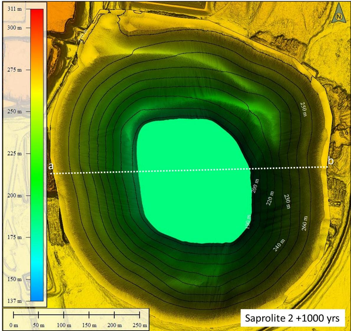
**Figure B 17:** Landform evolution model output after 1,000 years of the Wyoming 1 Pit with a Saprolite 2 surface in a bare (unvegetated) condition.
