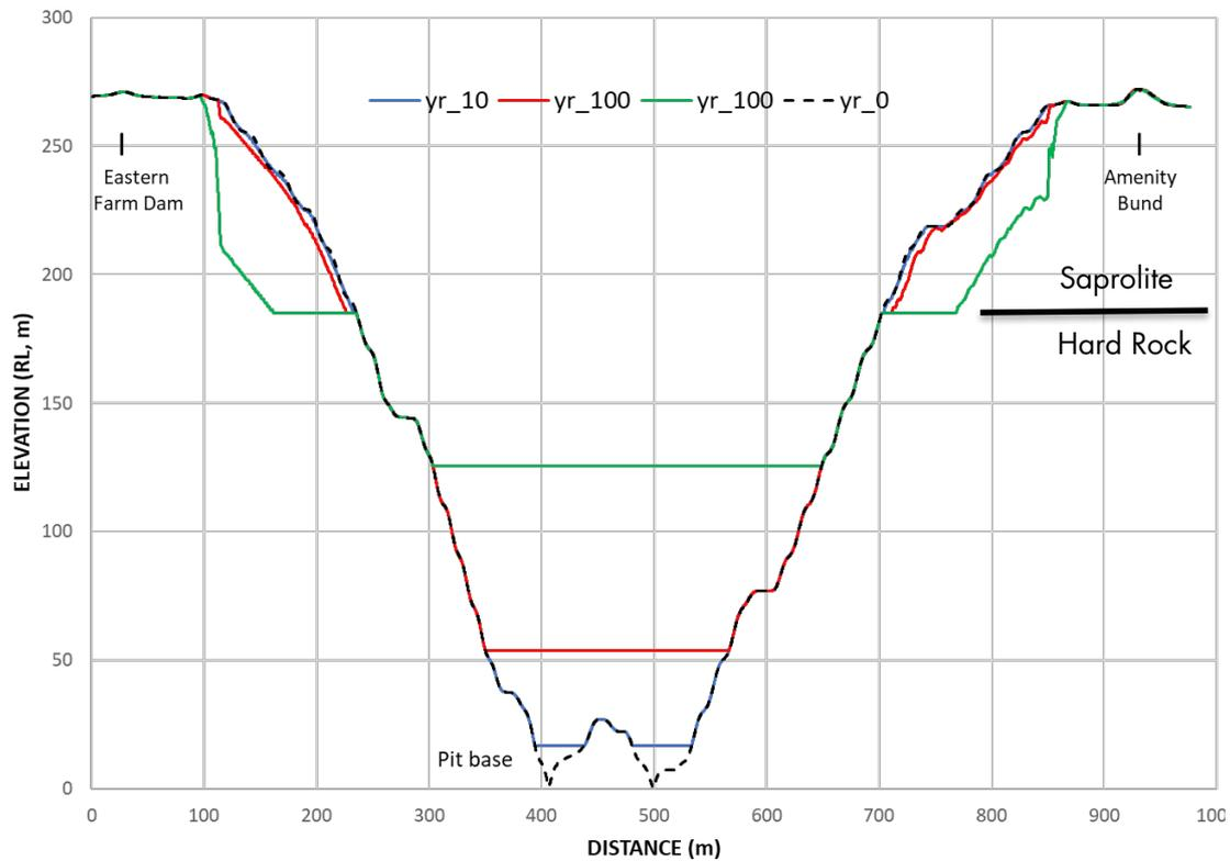
**Figure 11:** Conceptual representation of deposition levels of eroded sediment into SAR North Pit at time intervals of 10, 100, and 1,000 years.
