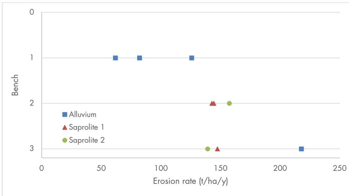
**Figure 3:** Erosion rates tend to increase with depth.
