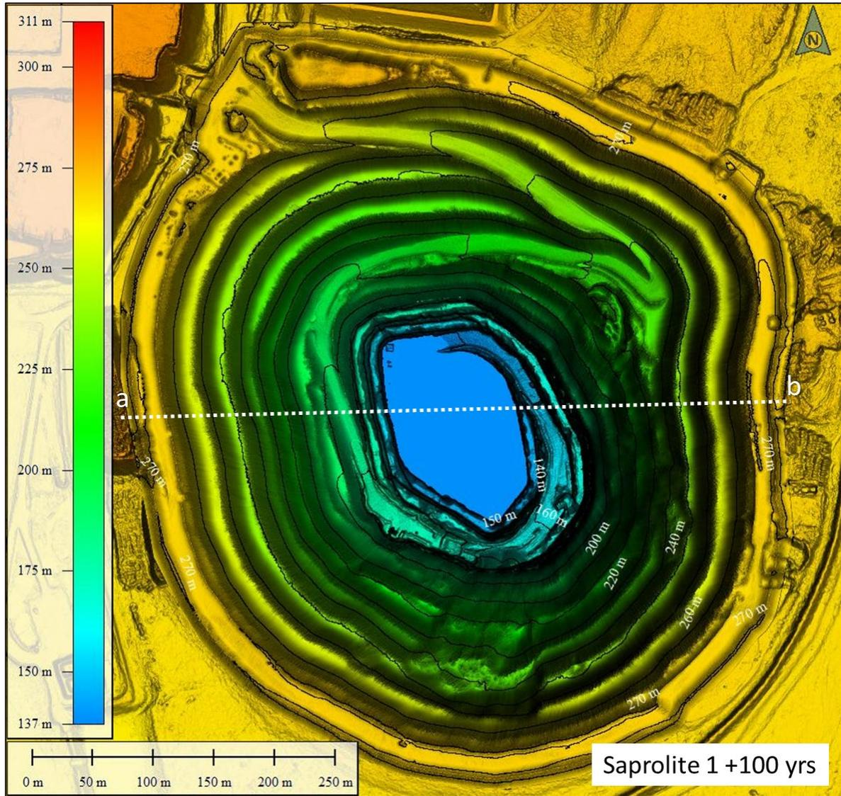
Figure B 9: Landform evolution model output after 100 years of the Wyoming One Pit with a Saprolite 1 surface in a bare (unvegetated) condition.
