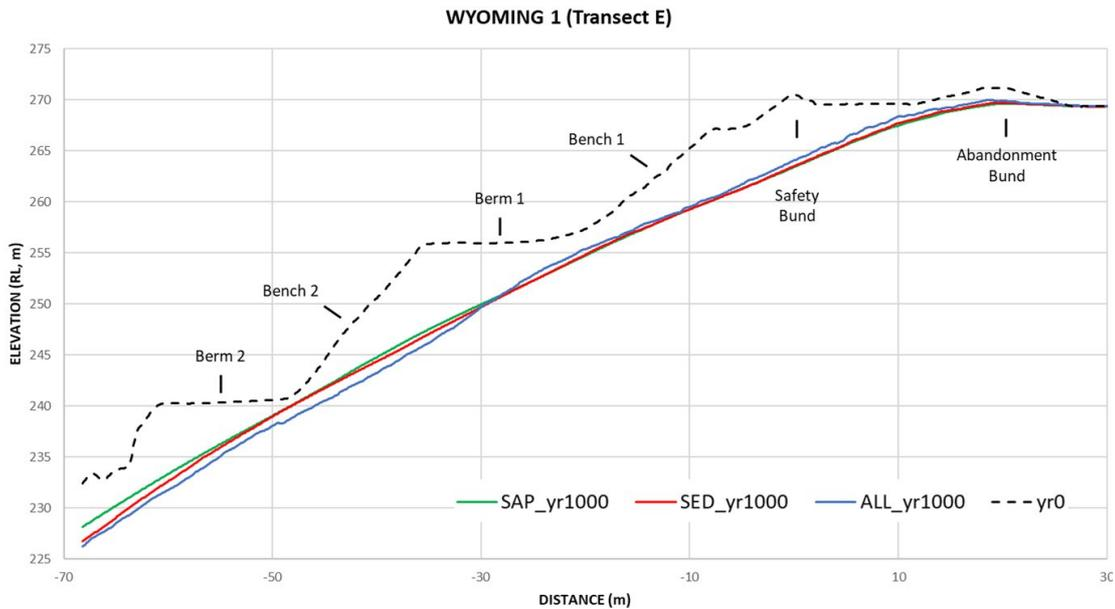
**Figure 4:** Comparison of predicted erosion of the Alluvial (All), Saprolite 1 (Sap1), Saprolite 2 (Sap2) lithologies of interest at 1,000 years.
