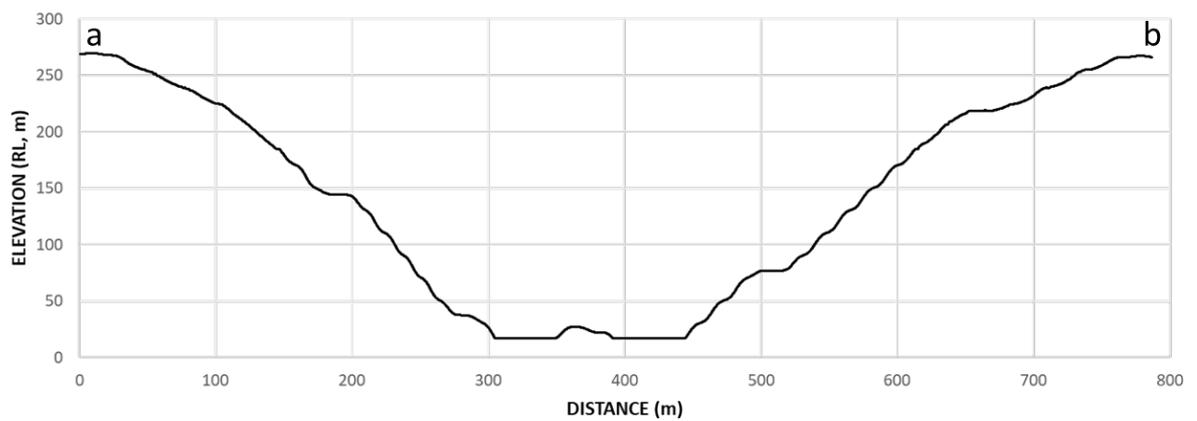
**Figure B 20:** Cross section of the transect in Figure B 19. Note the interface of the batters and berms is distinct and relatively sharp.
