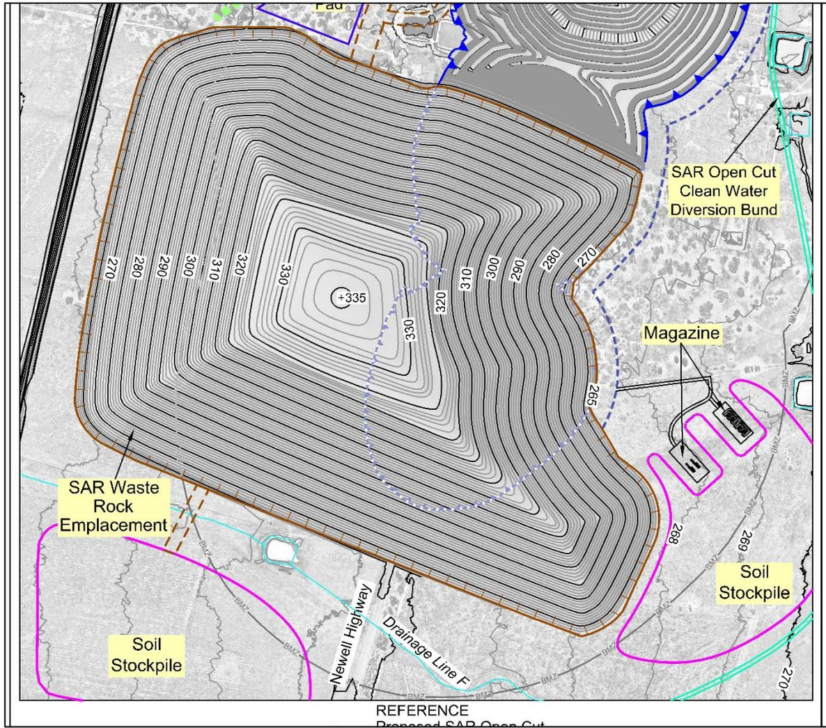
**Figure A 2.** Conceptual layout of the post-mining surface of the SAR North Pit. The current plan is for the two southern pits to be backfilled with waste rock, and the SAR North Pit will remain as a void (Courtesy RW Corkery, 2021).
