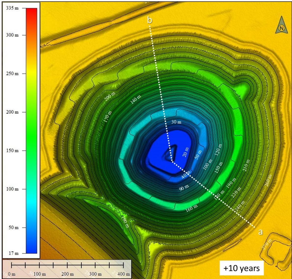
**Figure B 19:** Landform evolution model output after 10 years of the SAR North Pit with a Saprolite 1 surface in a bare (unvegetated) condition.
