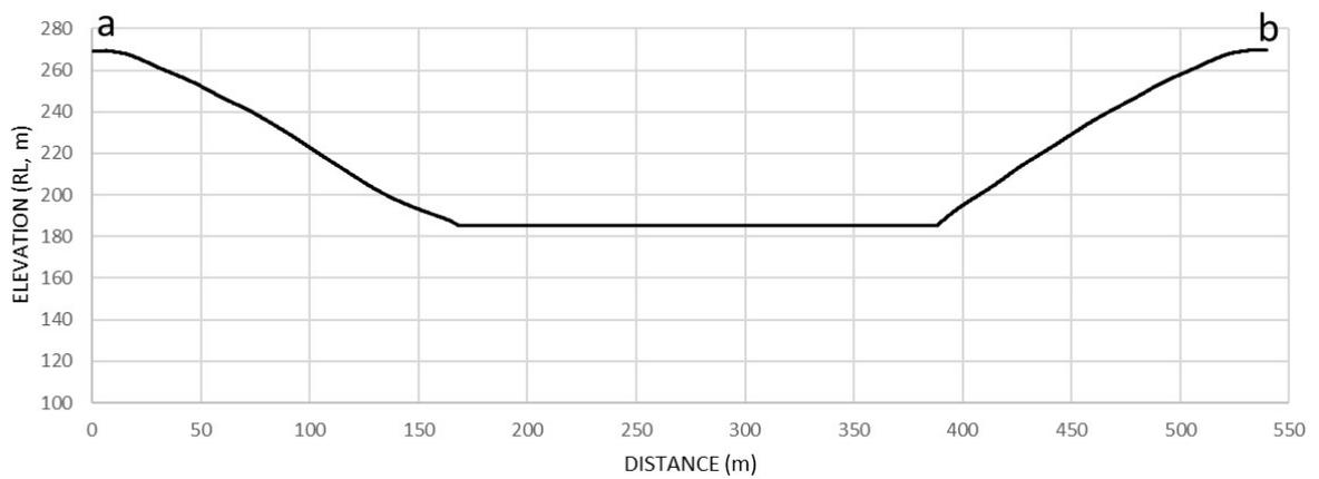
**Figure B 18:** Cross section of the transect in Figure B 17. Note the interface of the batters and berms is no longer detectable due to erosion of the pit wall.
