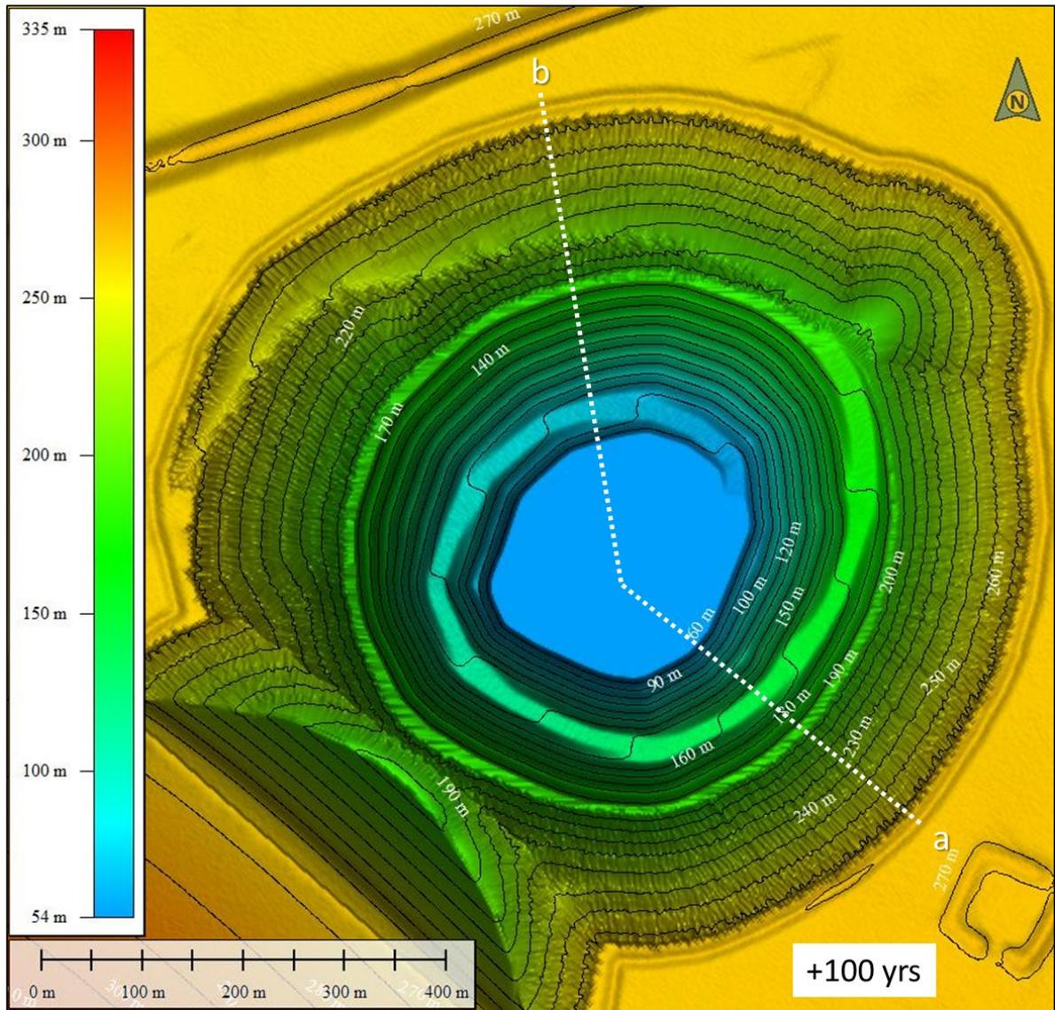
**Figure B 21:** Landform evolution model output after 100 years of the SAR North Pit with a Sapolite 1 surface in a bare (unvegetated) condition.
