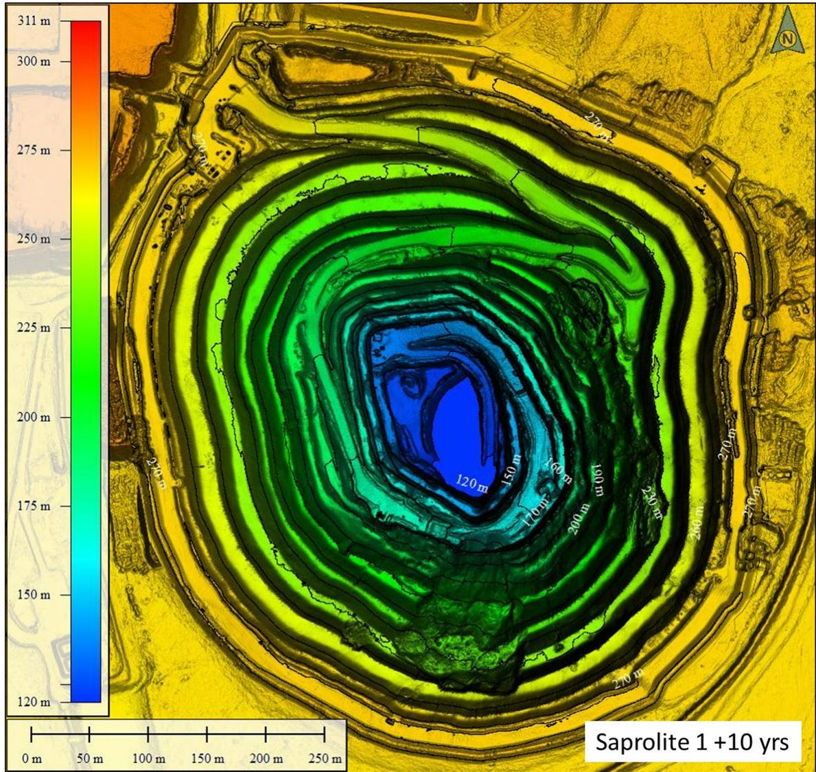
Figure B 7: Landform evolution model output after 10 years of the Wyoming One Pit with a Saprolite 1 surface in a bare (unvegetated) condition.
