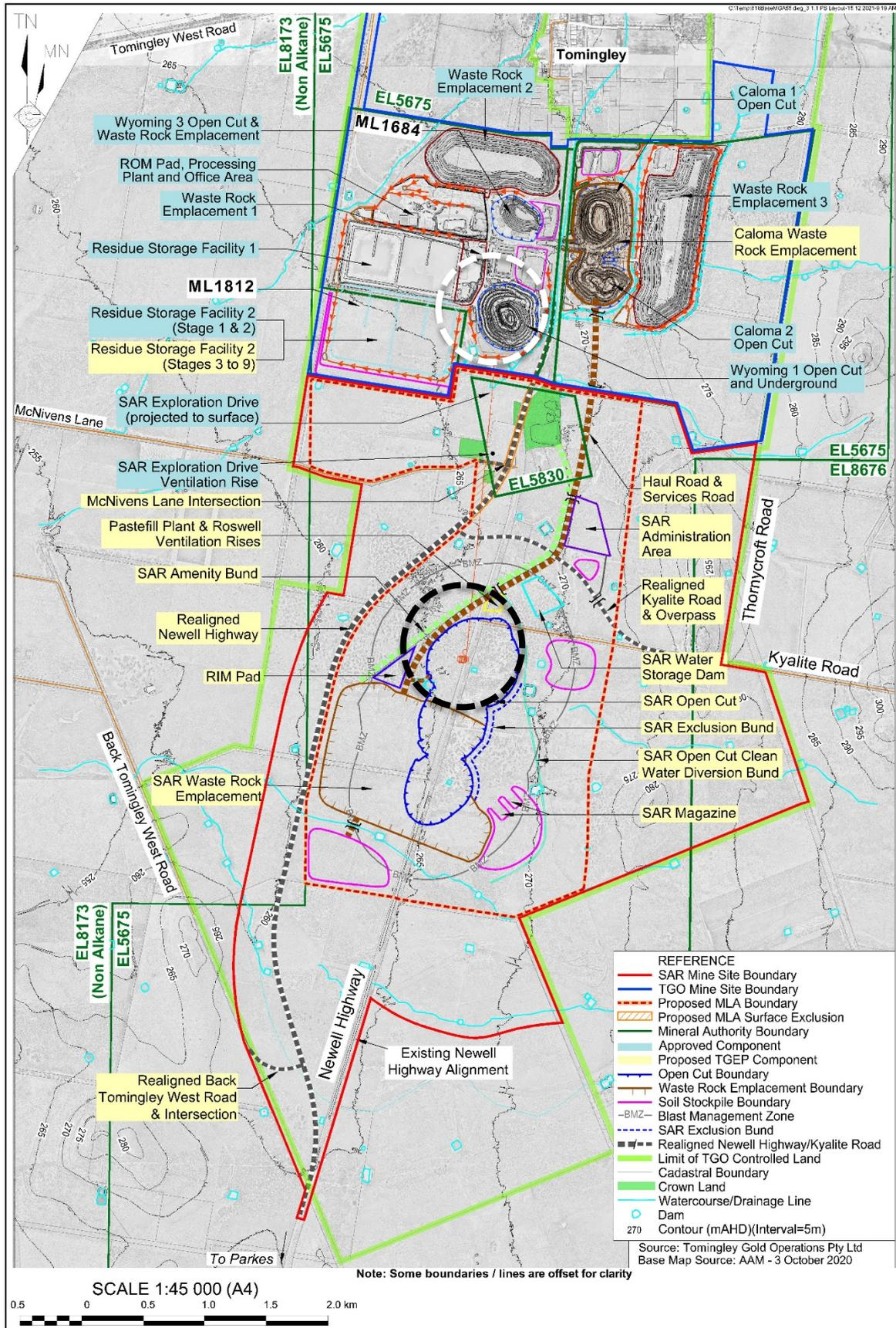
**Figure A 1.** General arrangement of the TGO and the TGE (Courtesy RW Corkery, 2021) with Wyoming 1 Open Cut (white dashed circle) and SAR North Pit (black dashed circle) highlighted.
