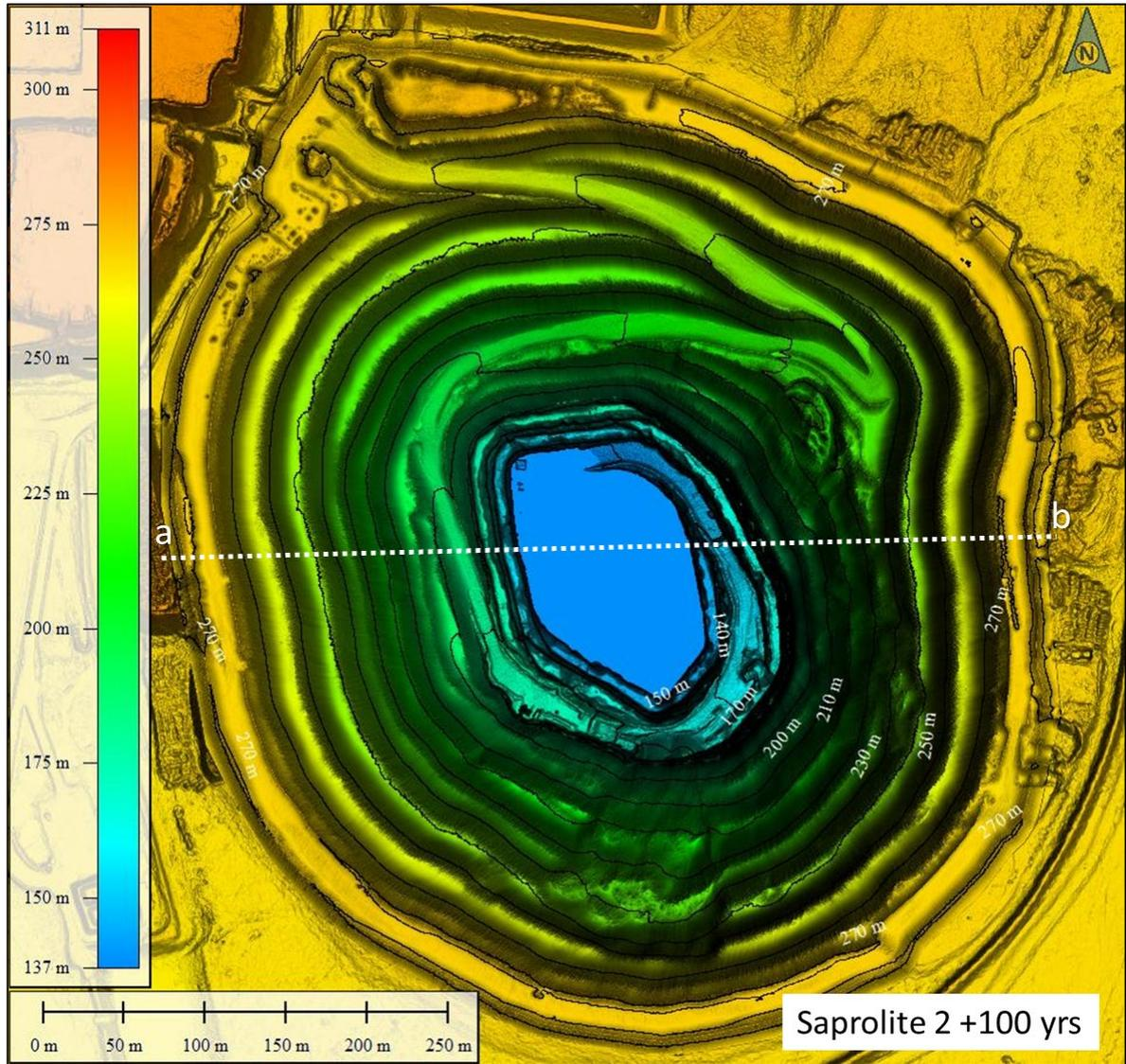
**Figure B 15:** Landform evolution model output after 100 years of the Wyoming 1 Pit with a Saprolite 2 surface in a bare (unvegetated) condition.
