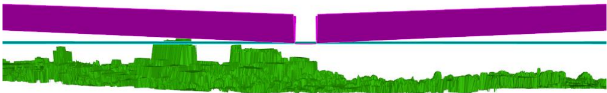
Figure 2: The VFR (magenta) and OIS (blue) surfaces above the modelled LiDAR data (green) 500 m either side of the HLS.
