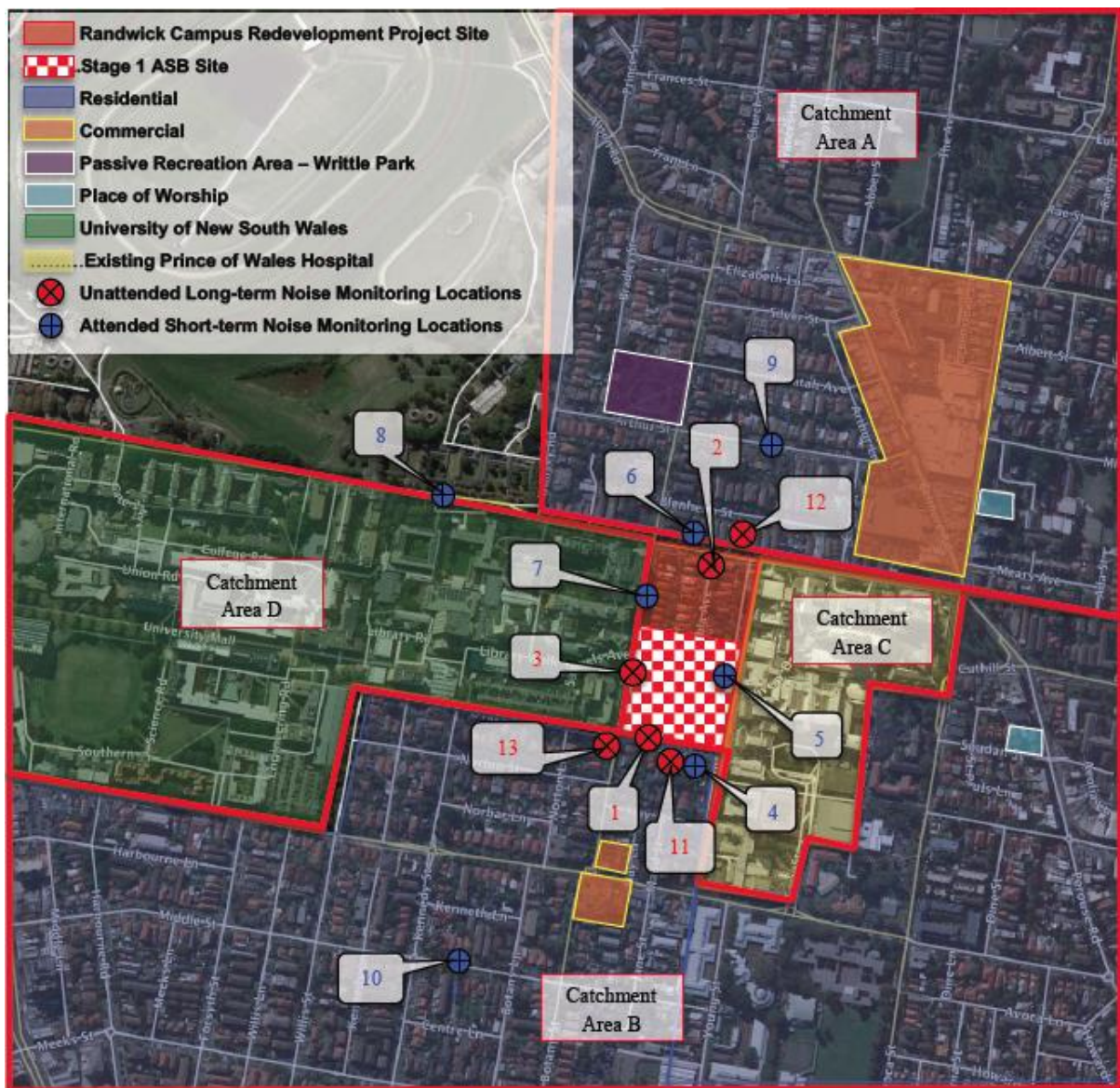
Figure 7-3 The site in relation to the location of noise-sensitive receivers. In addition to unattended long-term noise monitoring, attended short-term noise measurements were also carried out at Locations 1 to 3 (Source: Acoustic Studio, 2018).
