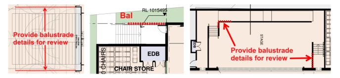
As the balustrades that protect the top of the retractable seating protect a fall of more than 4m the balustrade is not permitted to have any horizontal or near horizontal elements between 150 mm and 760 mm above the floor that facilitates climbing.
