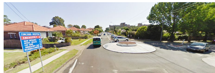
Corner Hospital Road / Nullawarra Avenue Directional sign is parallel with main traffic and not visible from the required distance
