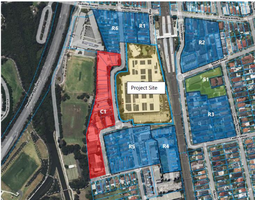
Figure 16 Surrounding Sensitive Noise Receivers
