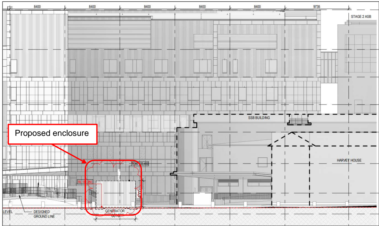
Figure 5 | West elevation of generator enclosure (Source: Jacobs)
