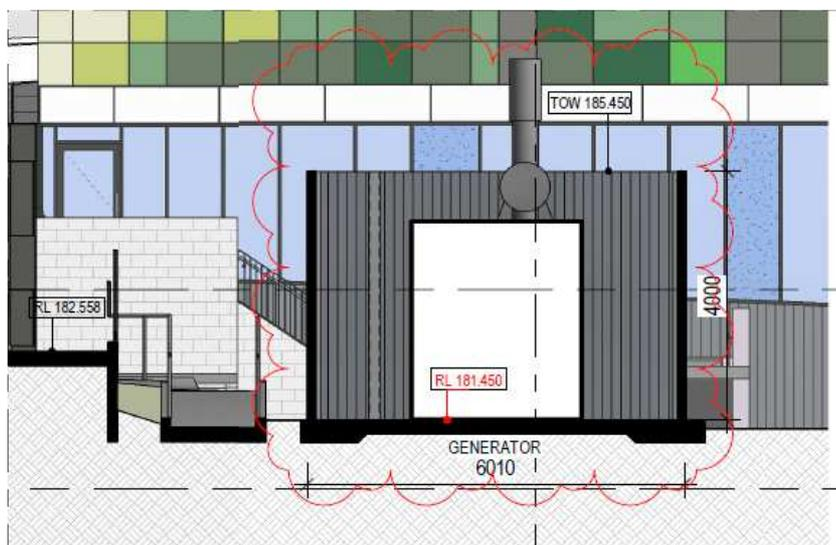
**Figure 3** Section view of the Generator enclosure (with generator in centre)
