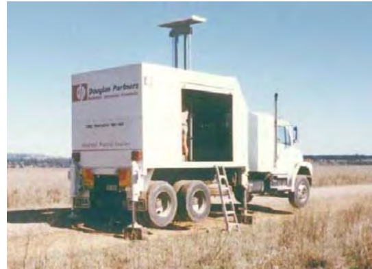
Figure 2: Purpose built CPT rig
