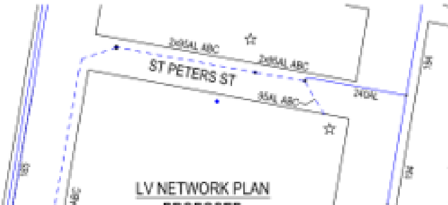
Figure 5 – Existing overhead electrical supply
