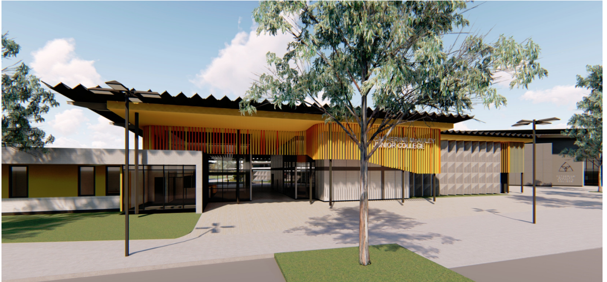
j. Final Design Image of the Primary School Entry/Admin/Hall. The controlled entry point allows passive surveillance of the School Entry, Carpark, Canteen, Library & Hall and facilitates after hours access to the Hall.
