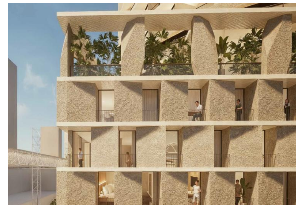
The building façade generally avoids heavy faces of glazing that reflect solar radiation to hard surfaces on the street below—non reflective façade finishes, and avoidance of glazed balustrading, help mitigate this effect
