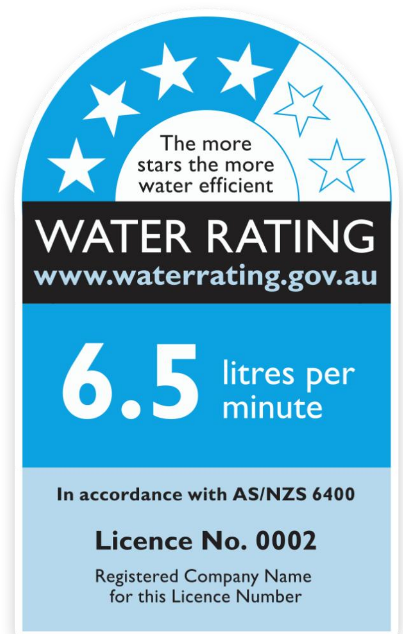
WELS shower label certifying 6.5 L flow rate—consistent with this proposal
