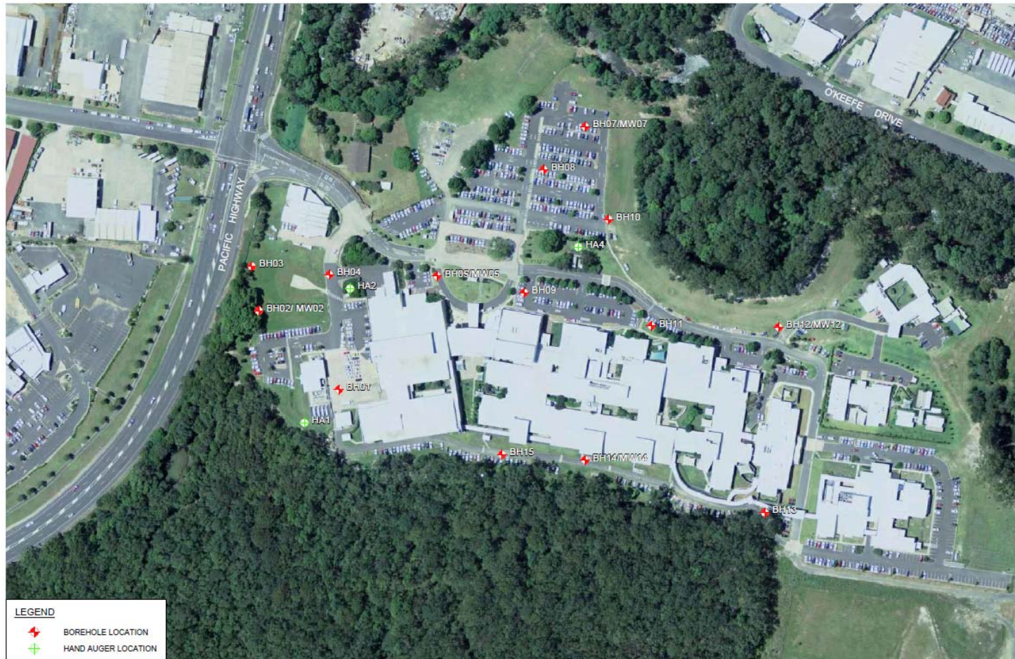
Plate 7-8 Sampling and Borehole Locations
