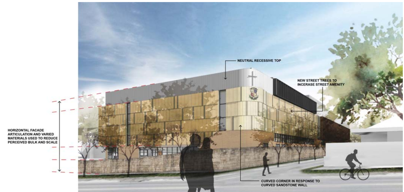
Figure 10 | Built Form and Facade Treatment at the intersection of Gladesville Road and Luke Street
