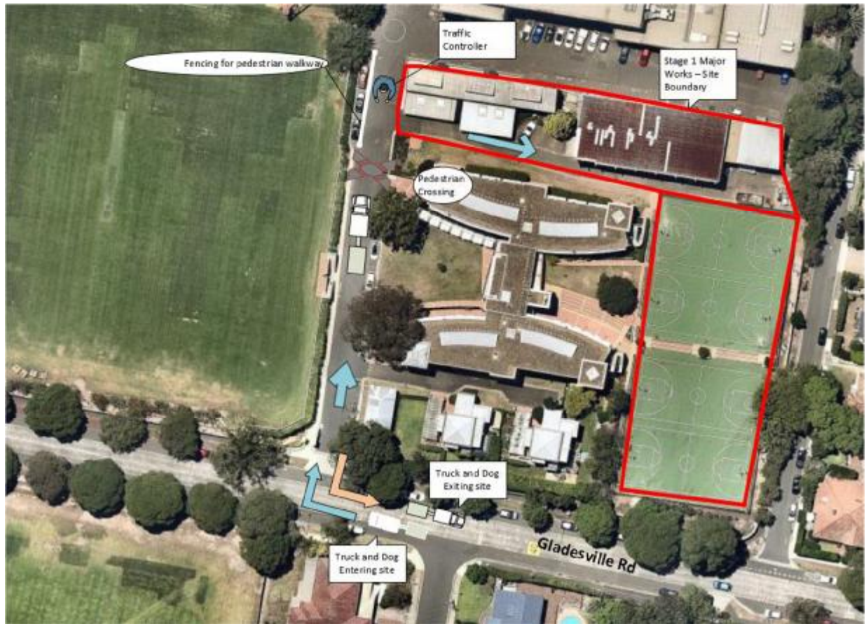
Figure 5. Site Access Route during demolition Phase
