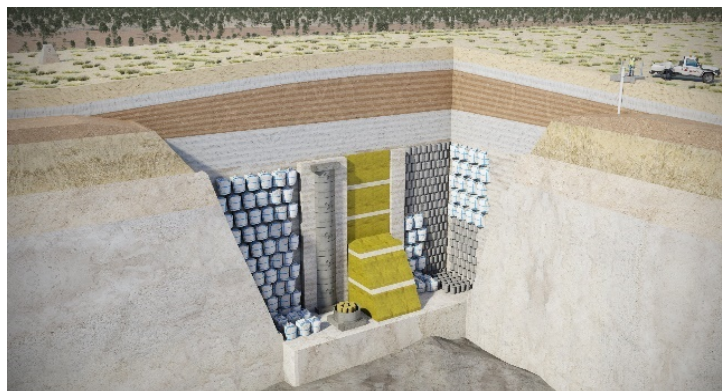
The space between the waste packages would be filled with clay or cement and compacted to remove air and void space, until approximately six to 12 metres below the existing ground surface.
