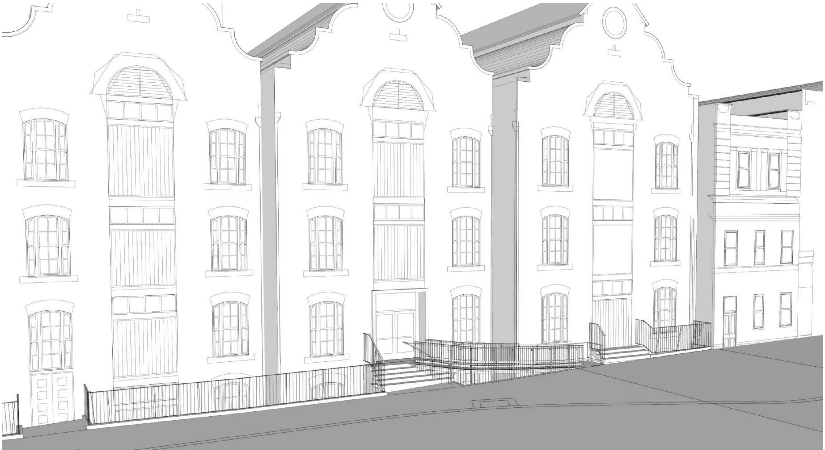
View from the street demonstrating the retention of the existing steps into Bay 4 and views to the façade below the ramp.
