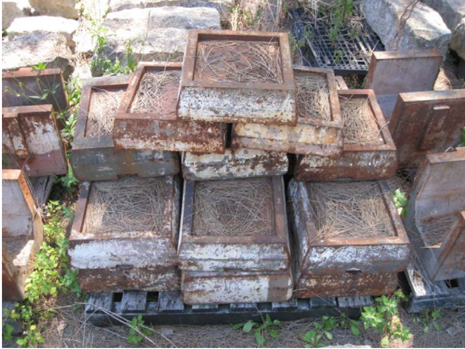
11. Steel collar bottom pieces. Note: stacked upside-down.
