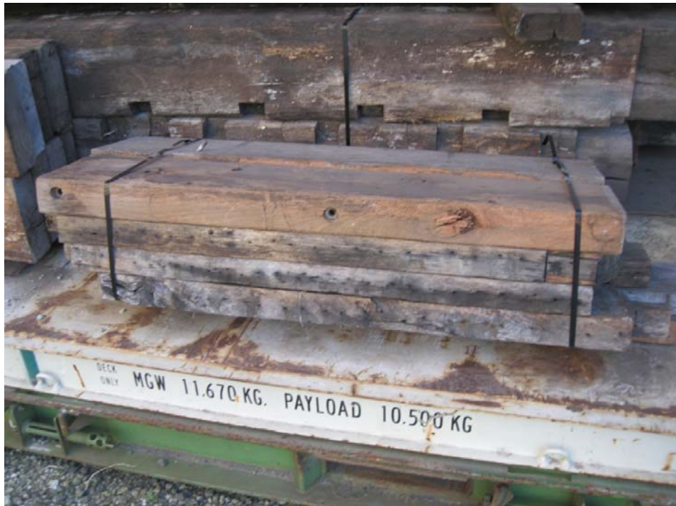
6. 5. Suspected sections of timber joists cut into shorter segments. Stored in NW container.
