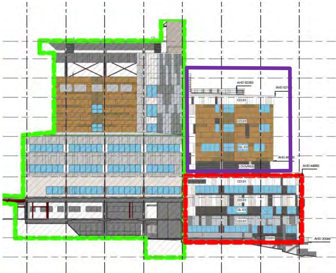
Figure 12: Proposed eastern elevation of the northern and southern towers, showing the existing southern tower (green), to be constructed and approved northern tower ((red), and the proposed addition (purple). (Source: Conrad Gargett, East West Elevations, drawing no. DA30002, revision A, 6 April 2018)
