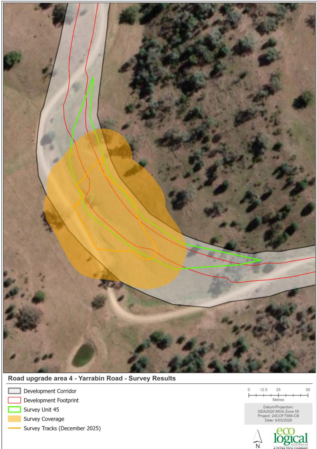
Figure 50: Survey coverage and results – road upgrade area 4
