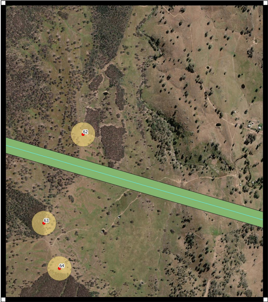
Figure 4: WTG 62 envelope based on 180 m rotor diameter, relative to 0.6 multiplied by maximum 1 st Fresnel Zone extent of Link 1.
