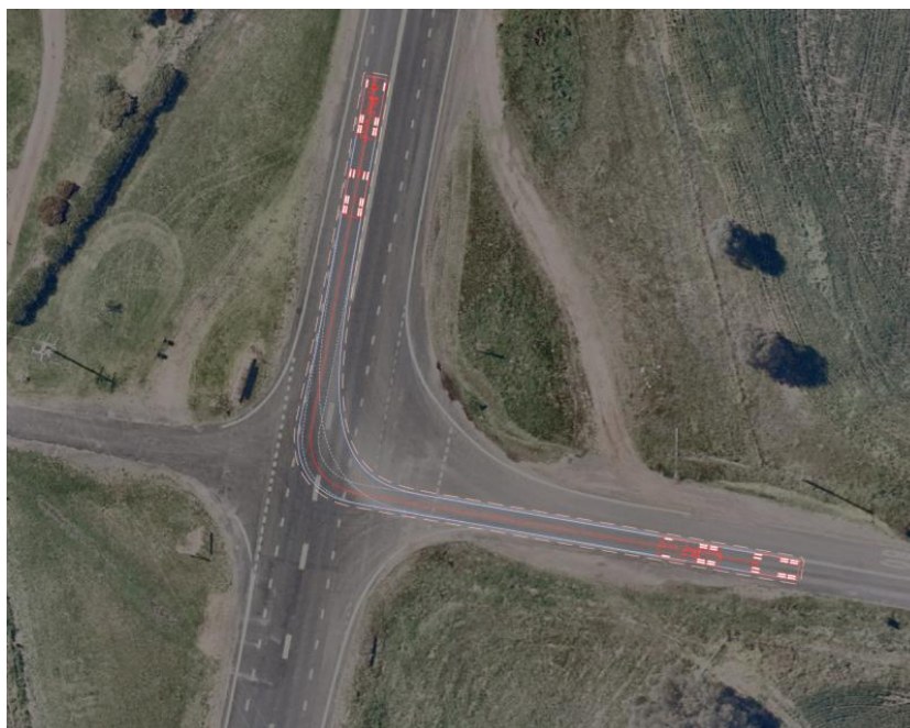
Figure 2: 19m truck-and-dog right turn swept path from Burrendong Way into Mitchell Highway
