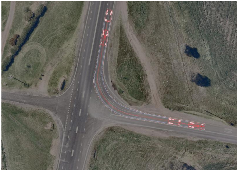
Figure 2: 19m truck-and-dog right turn swept path from Burrendong Way into Mitchell Highway
